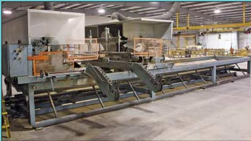
Clary Five-Blade Truss Component Saw
