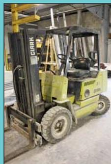
2,750 Lb. Clark GPX-20 Pneumatic Tire LP Gas Lift Truck
