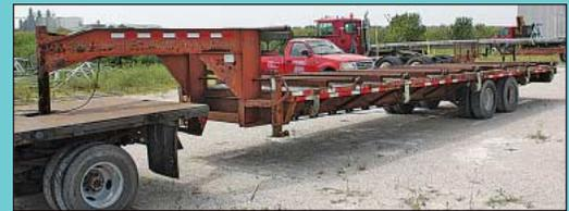
40' Mfg. Unk. Gooseneck Roller Bed Truss Trailer
