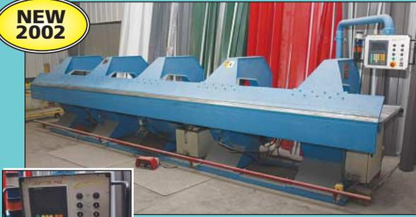
21' Jorns AG Norma-Line-125S-SO-CNC 400A-6.4HS Power Panel Bending Machine
