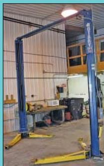
9,000 Lbs. Cap Rotary Lift Model SPOA9N300 Floor Mounted Hydraulic Vehicle Lift
