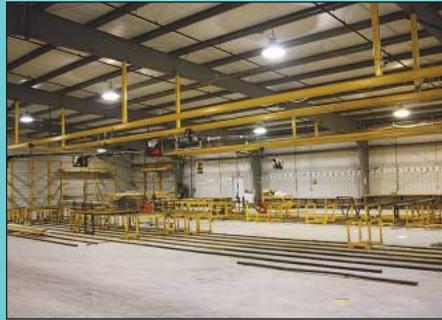
(2) 15' Wide X 80' Long Manual Overhead Bridge Type Truss Assembly Lines
