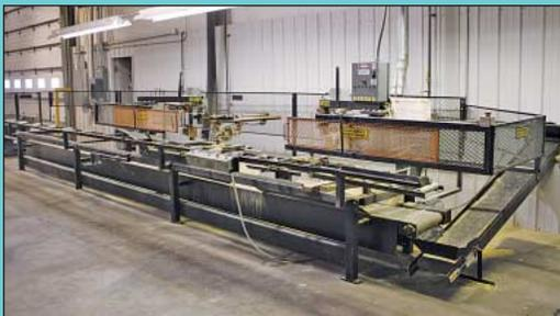
Fast Cut Four-Blade Truss Component Saw
