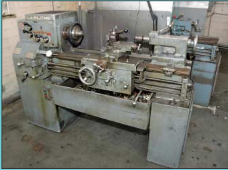
15" X 30" Leblond Regal Geared Head Engine Lathe
