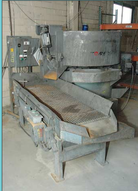
(1 of 2) Torex Model T-6026-F Vibratory Bowl Type Finishing Machine
