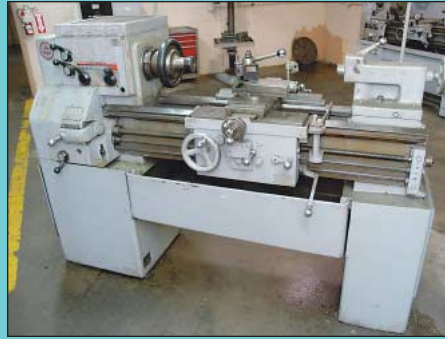
15" X 30" Leblond Dual Drive Geared Head Engine Lathe
