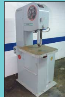
16" DoAll Model 1611-U Vertical Band Saw
