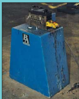
2" PA Industries Model PSS-29D Straightener
