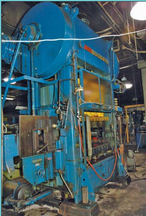
200 Ton Niagara Model BP2-200-60-42 Variable Speed Straight Side Double Crank Press
