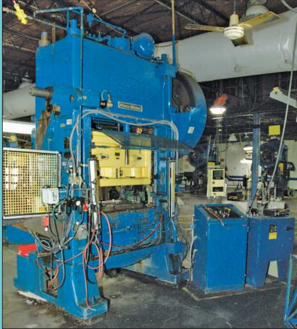
(2) 100 Ton Minster Model P2-100-48 Piece-Maker Variable Speed Straight Side Double Crank Presses
