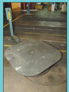
(2) 5,000 LB X 48" Coil Mate Model EZ5048 Horizontal Coil Reels
