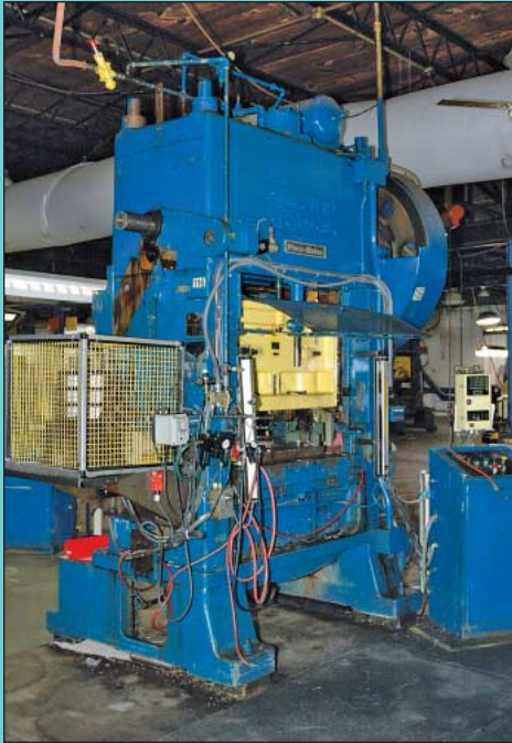
(2) 100 Ton Minster Model P2-100-48 Piece-Maker Variable Speed Straight Side Double Crank Presses
