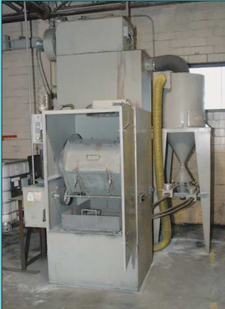
2 Cubic Foot Blast-It-All Model TBS2RPJT-3 Cabinet Type Tumbling Barrel Parts Deburring Machine
