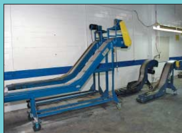
(6) 8" X 84" Livonia Magnetics Model B-11 Magnetic Belt Incline Portable Scrap Conveyors
