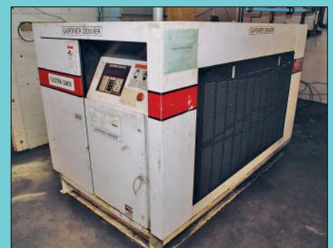
100 HP Gardner Denver Model EAPOMB Cabinet Type Rotary Screw Air Cooled Air Compressor
