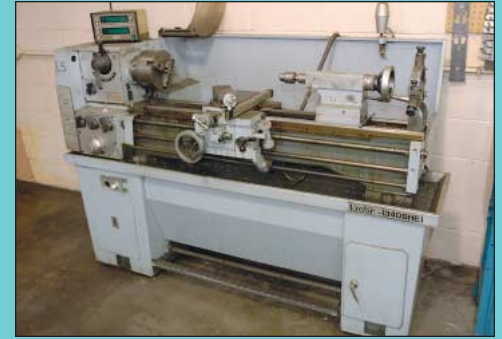
13" X 40" Victor Model 1340GHE Geared Head Engine Lathe
