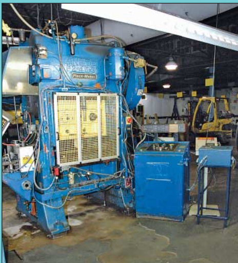
45 Ton Minster Model P2-45-36 Piece-Maker Variable Speed Straight Side Double Crank Press
