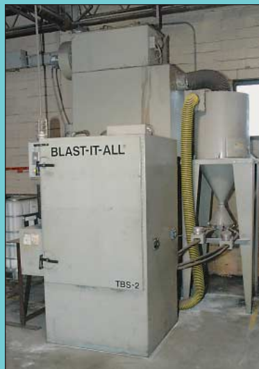
2 Cubic Foot Blast-It-All Model TBS2RPJT-3 Cabinet Type Tumbling Barrel Parts Deburring Machine
