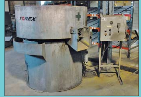
(2 of 2) Torex Model T-6026-F Vibratory Bowl Type Finishing Machine
