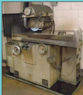
6" X 18" Thompson Hydraulic Surface Grinder
