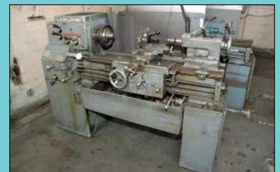
15" X 30" Leblond Regal Geared Head Engine Lathe
