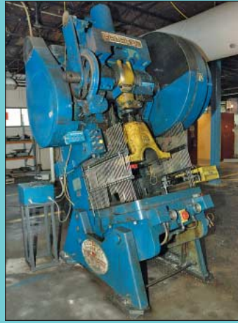
80 Ton Federal Model F7 Flywheel Type OBI Press
