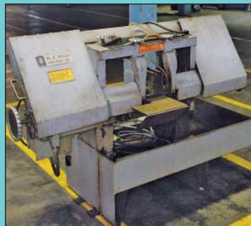
10" X 16" W.F. Wells Model L-10 Twin Post Horizontal Band Saw
