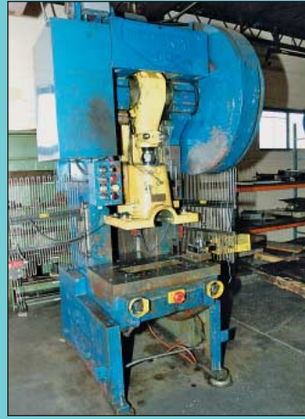
60 Ton Federal Model 60 Flywheel Type OBI Press
