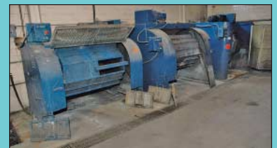
(5) 30" X 48" Rampart Model HT3048 Twin Compartment Tumbling Barrel Parts Deburring Machines
