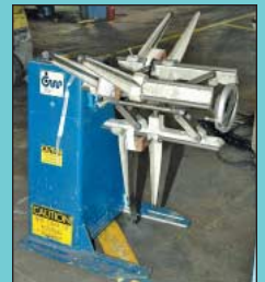
1,600 LB X 18" CWP Model 2R Single End Coil Reel
