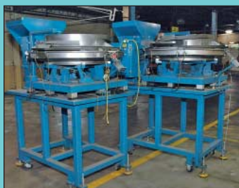
(2) 30" Dia. Fortville Vibratory Parts Feeders w/ Loading Hoppers
