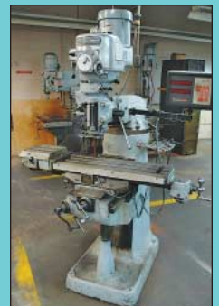
1-1/2 HP Bridgeport Variable Speed Vertical Milling Machine
