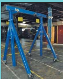
2,000 LB T&S Portable Adjustable Height A-Frame Gantry Crane
