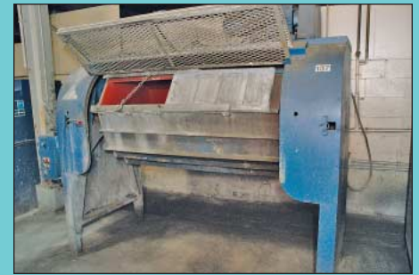
(4) 32" X 60" Rampart Model HT3260 Twin Compartment Tumbling Barrel Parts Deburring Machines
