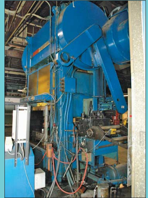
200 Ton Niagara Model BP2-200-60-42 Variable Speed Straight Side Double Crank Press
