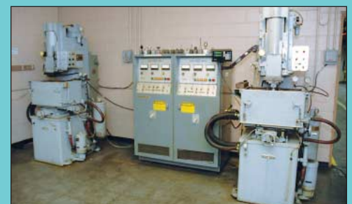
Bank View (2) Cincinnati Ram Type EDM Machines
