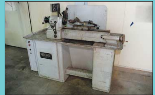
9" X 18" Hardinge Dovetail Toolroom Engine Lathe
