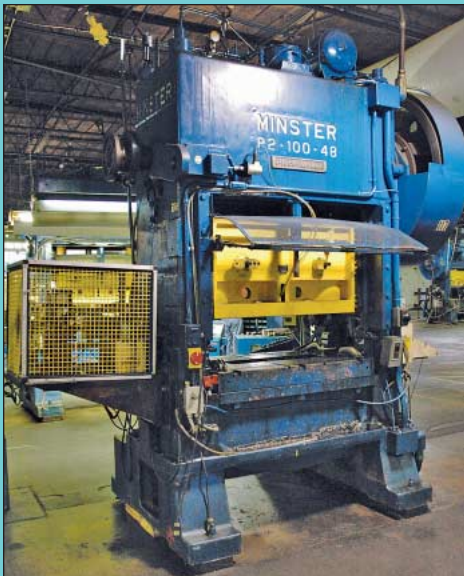
(2) 100 Ton Minster P2-100-48 Piece-Maker Straight Side Double Crank Variable Speed Presses
