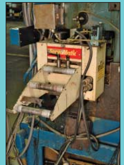
6" Servomatic Servo Feed
