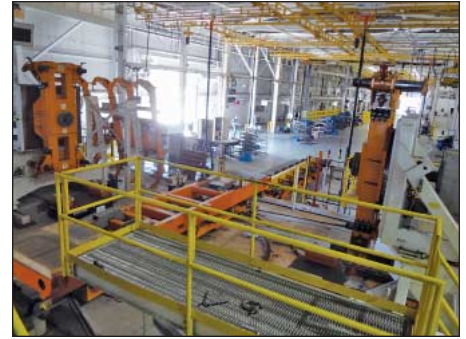
(2) 34,000 Lb. (Approx.) Vehicle Rotators
