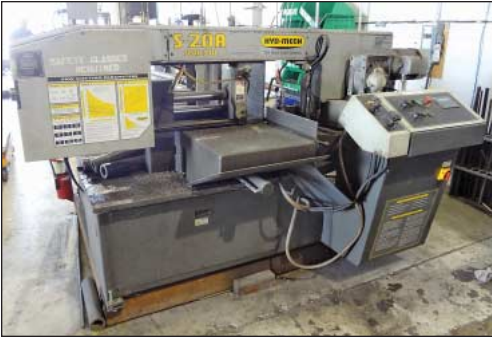
14" X 20" Hyd-Mech Model S-20A Series III Automatic Miter Base Horizontal Band Saw
