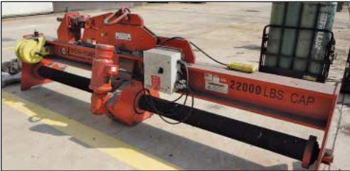
22,000 Lb. Capacity Caldwell Model 22LS-150 Post-Turner
