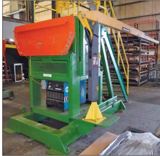
(3) 6,800 Lb. Capacity Headstock / Tail Stock Welding Assembly Stations with Hydraulic Driven Headstocks
