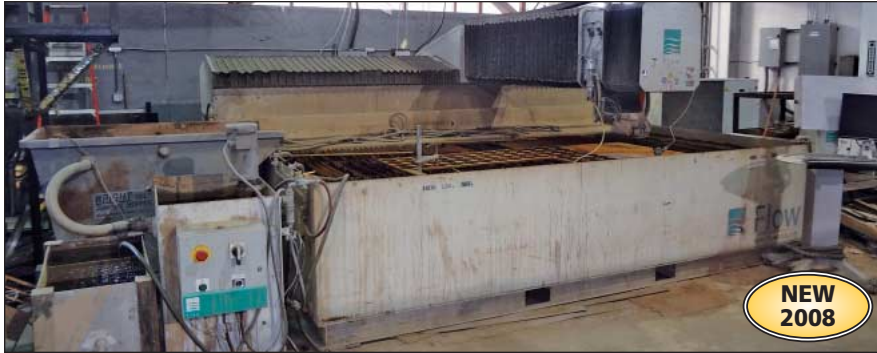
Flow Jet Model 87K Traveling Head CNC Water Jet Cutting Machine
