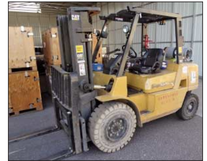
8,000 Lb. Caterpillar Model GP40K1 Pneumatic Tire LP Gas Lift Truck
