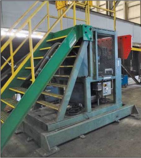
(3) 6,800 Lb. Capacity Headstock / Tail Stock Welding Assembly Stations with Hydraulic Driven Headstocks
