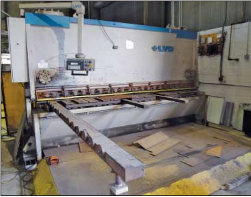
1/2" X 14' LVD Model 130H75-MNC CNC Hydraulic Power Squaring Shear
