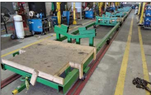
Large Quantity Heavy Steel Welding, Assembly and Transport Fixtures
