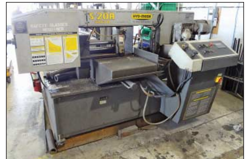
14" X 20" Hyd-Mech Model S-20A Series III Automatic Miter Base Horizontal Band Saw
