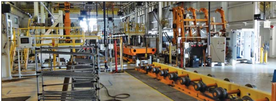
50'W X 400'L Large Vehicle Assembly Line – (57) Spanco Bridges, 25 Ton Lift and 17 Ton Rotator
