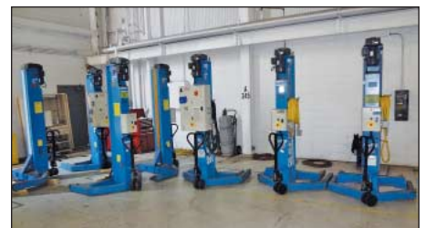
(8) 16,000 Lb. Sefac Model 1600M72 Electric / Hydraulic Vertical Type Vehicles Jacks
