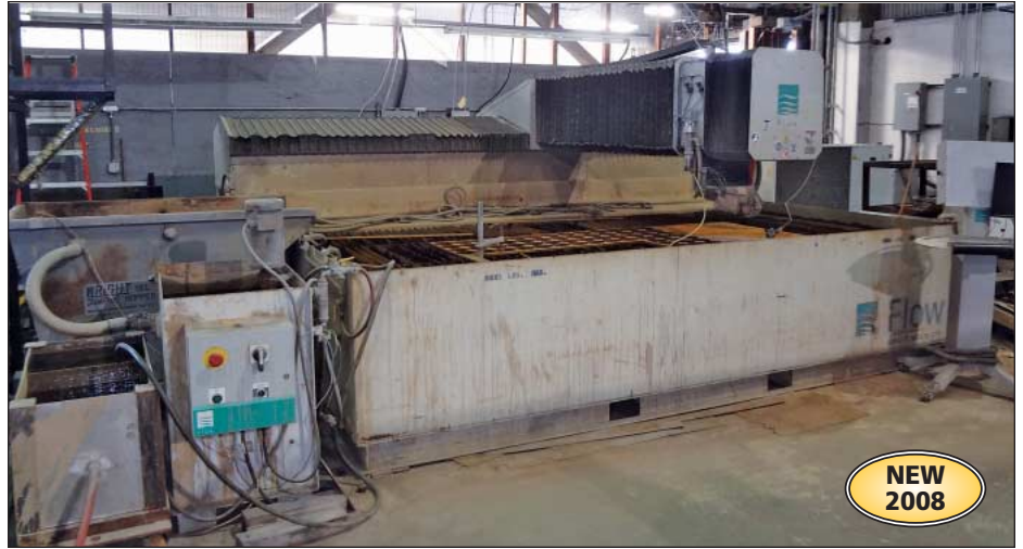
Flow Jet Model 87K Traveling Head CNC Water Jet Cutting Machine
