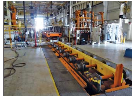
57,000 Lb. Capacity Autoquip Scissor Lift Table w/ 40" X 18' Long Platform and 25' Long Vehicle Exit Fixture
