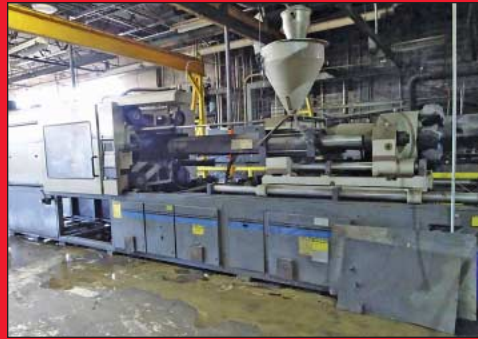
500 Ton x 85 Oz. Cincinnati Milacron Model VH500-85 Hydraulic Clamp Plastic Injection Molding Machine
