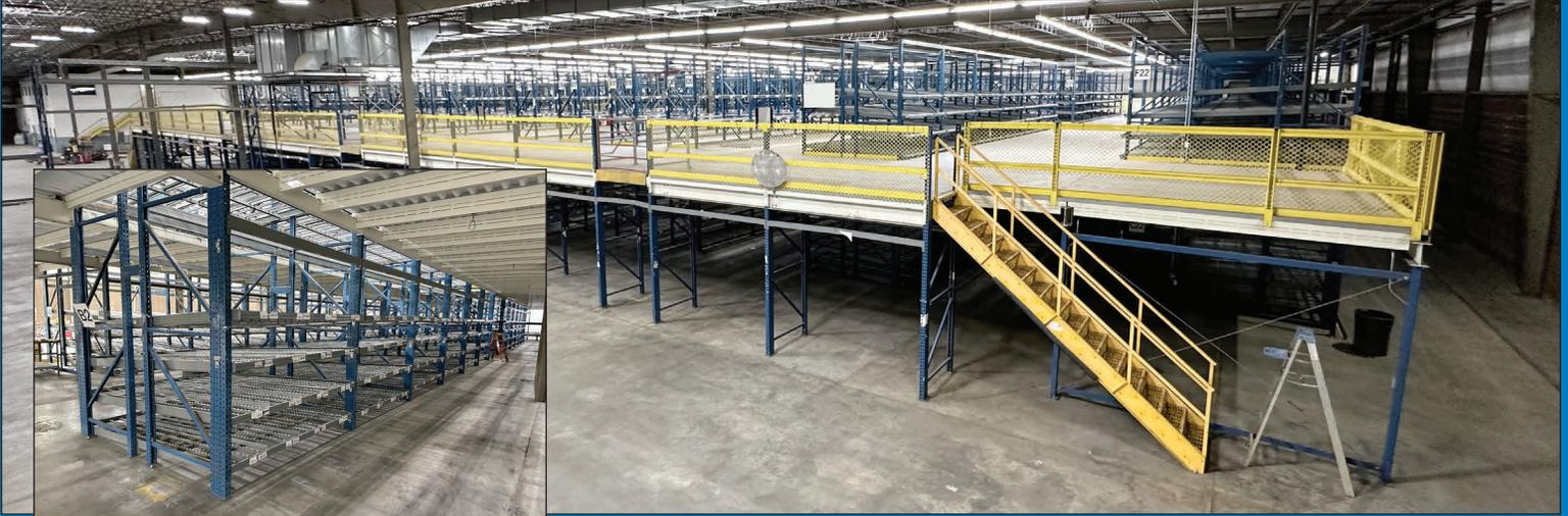
150' x 140' Two-Level Pick Module, Teardrop Upright and Beams
