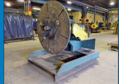
7,500 Lb. Pandjiris Model 75MVRMT Tilting and Rotating Welding Positioner
