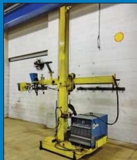
12' x 8' Pandjiris Model 61-M Welding Manipulator w/ Subarc DC-1000 Power Supply
