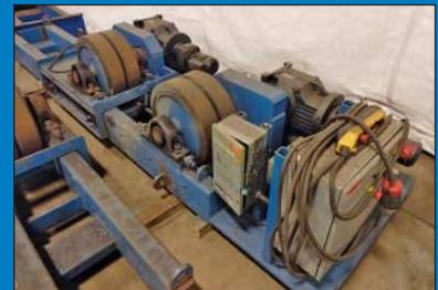
60 Ton IRCO Model 60TON Motorized Tank Turning Roll Set w/ Idler
