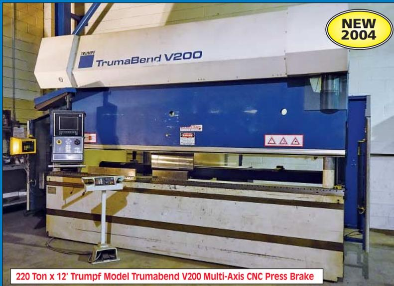
220 Ton x 12' Trumpf Model Trumabend V200 Multi-Axis CNC Press Brake
