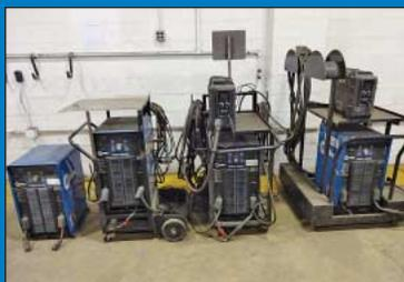
(4) 450 Amp Miller Pipe Pro 450RFC Welders w/ Model Pipe Pro 12RC Suitcase Wire Feeds
