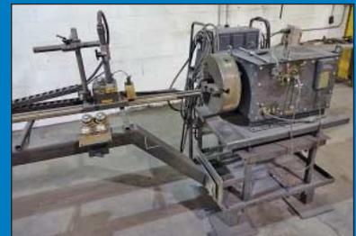
Bug-O Model SEC-1590-E Saddle and Elbow Plasma Pipe Beveling Machine
