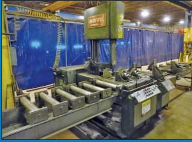
18" x 20" Marvel Model 81A Tilt Frame Automatic Vertical Band Saw
