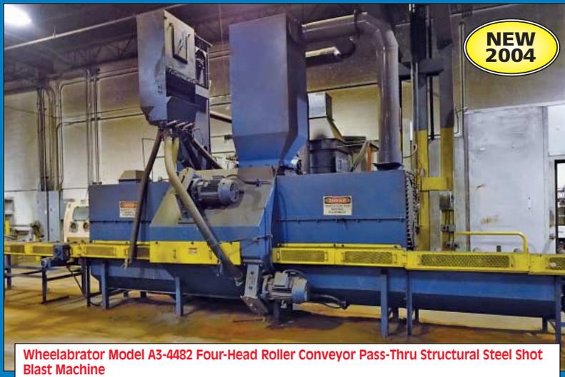
Wheelabrator Model A3-4482 Four-Head Roller Conveyor Pass-Thru Structural Steel Shot Blast Machine
