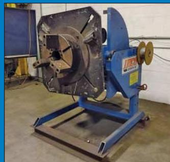
3,000 Lb. Irco Model 3K Tilting and Rotating Welding Positioner
