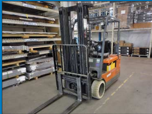
3,500 Lb. Toyota Model SFBE20 Electric Three-Wheel 36-Volt Lift Truck
