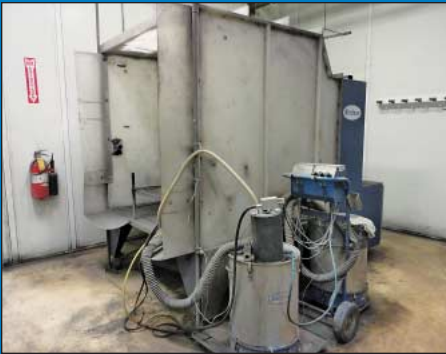
Nordson Model NVC-2 Econo Coat Series II Back Draft Powder Coat Booth
