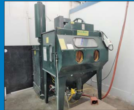
36" X 48" Maxi-Blast Model MB4836PDH-DC200 Plastic Blast Media Cleaning System
