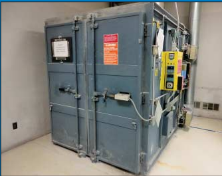
Controlled Pyrolysis Model PTR1503866 Natural Gas Cleaning Furnace
