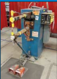
75 KVA Peer Model AR475 Rocker-Arm Spot Welder
