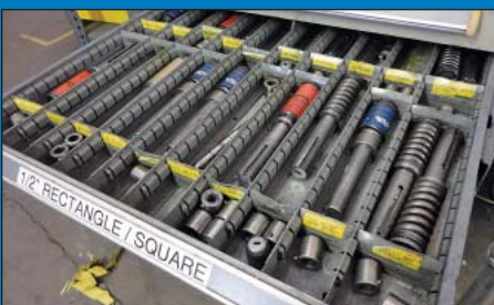
Large Quantity of Amada & Wilson Thick Punch Tooling Including Obround, Round, Rectangle, Etc. Punches
