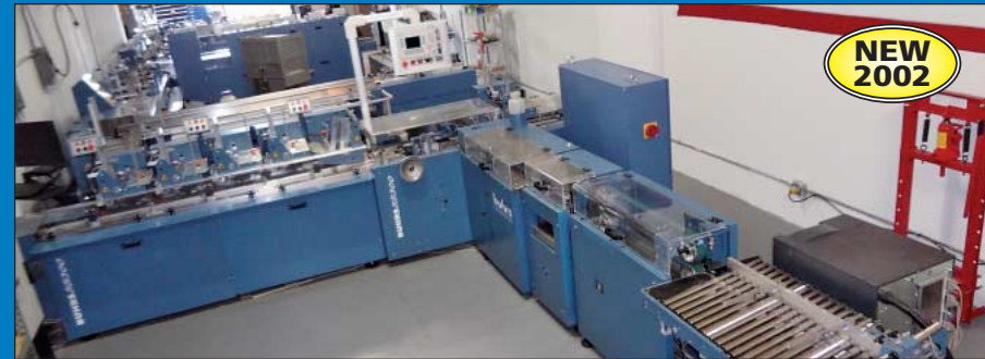
Buhrs Model BB300 Six-Station Automatic Inserting System w/ Scitex Printer and Lake Image Camera
