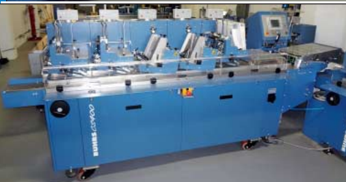
Buhrs Model CS400 Sidestreet Gathering Section BB700 without the Inserting Station
