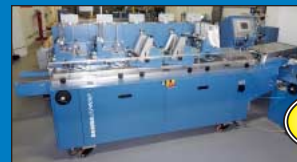
Buhrs Model CS400 Sidestreet Gathering Section BB700 without the Inserting Station
