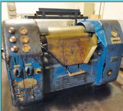
Cox Model 654 Hydramatic Triple Roller Mill
