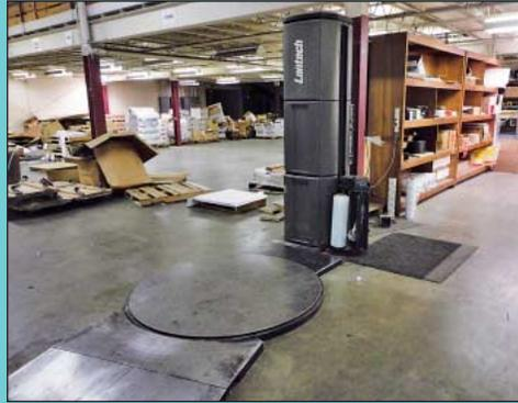
60" Lantech Q-Series Model 300 Rotary Stretch Wrapper
