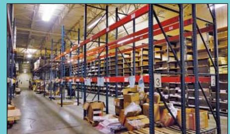
(56) Sections 42" Deep X 144" Wide X 16' High Adjustable Beam Pallet Racking, 3" X 3" Uprights
