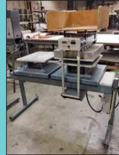
7) 16" X 20" Practix Model OK375 Shuttle Heat Transfer Presses
