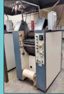
2) 16" Wide Astechnologies Model 7616 Narrow Web Drum Heat Transfer Machines
