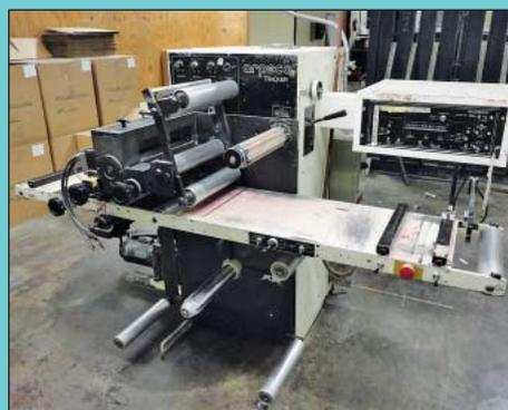
13" Arpeco Model Tracker Slitter / Rewinder
