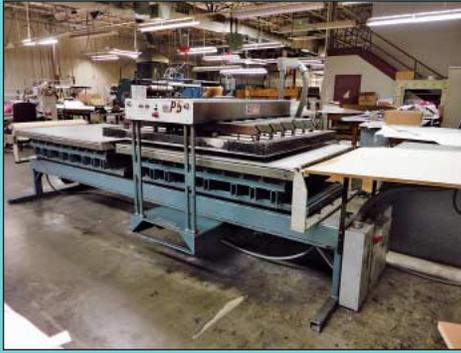
3) 42" X 66" Practix Model OK450 Shuttle Heat Transfer Presses
