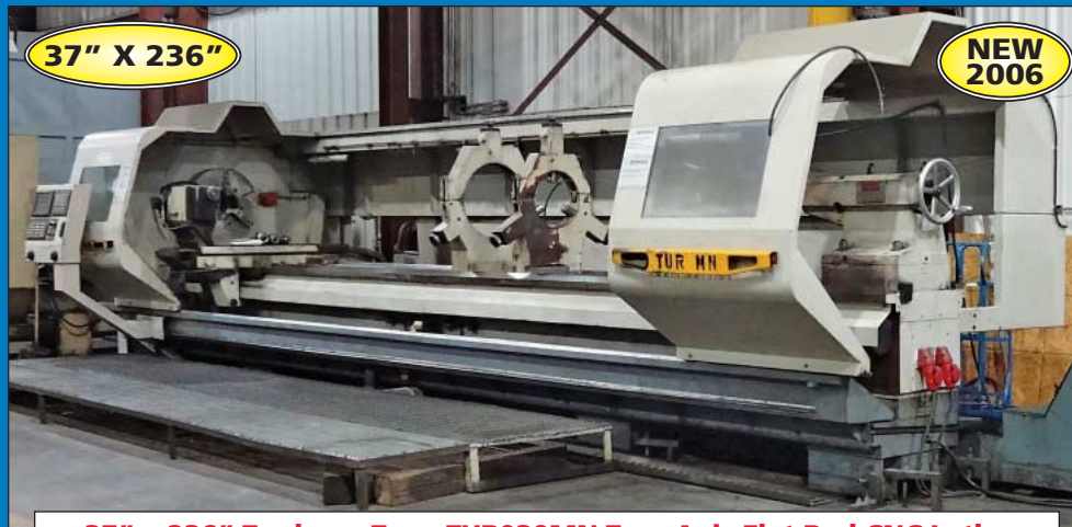
37" x 236" Toolmex Type TUR930MN Two-Axis Flat Bed CNC Lathe
