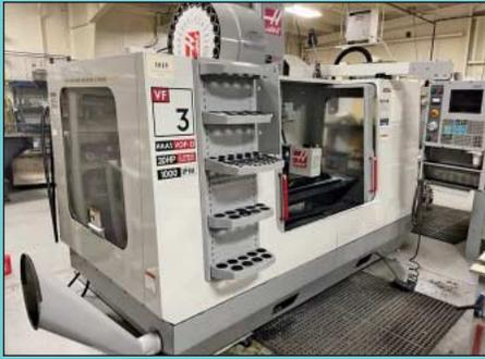
Haas Model VF-3B CNC VMC
