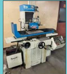
10" x 22" Supertec Model STP-1022ADC Surface Grinder
