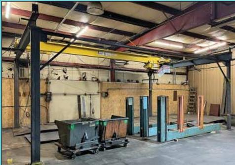
5 Ton x 29' Approx. Span x 19'L x 12'H Acco Single Girder Freestanding Bridge Crane
