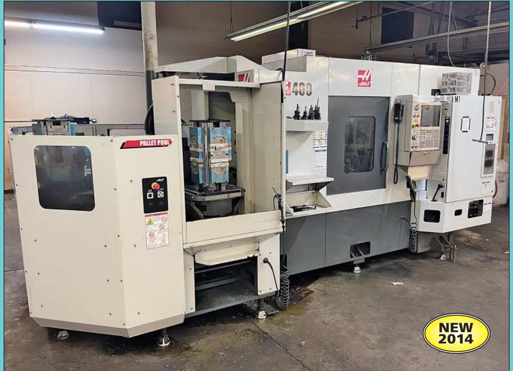
Haas Model EC-400PP CNC HMC with (6) Station Pallet Changer
