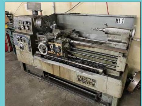
16" x 43" Supermax LG-1643 Gap Bed Engine Lather with DRO
