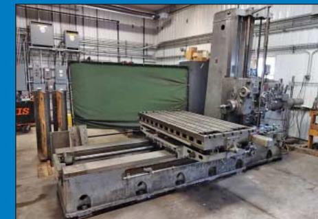
3" Giddings and Lewis Model 340-T Table Type Horizontal Boring Mill
