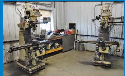
(2) 3-HP Jet Model JTM-4VS Vertical Milling Machines
