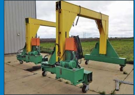
(2) Approx. 10 Ton Shop Built Heavy Duty Portable Hydraulic Gantry Units
