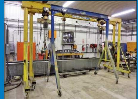
(2) 2 Ton x 16' Span Contrx Model GL-16 Portable A-Frame Gantry Cranes
