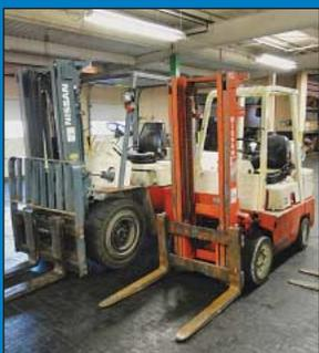
Bank View 9,000 Lb. Nissan Pneumatic Tire and 6,000 Lb. Nissan Solid Tire Lift Trucks
