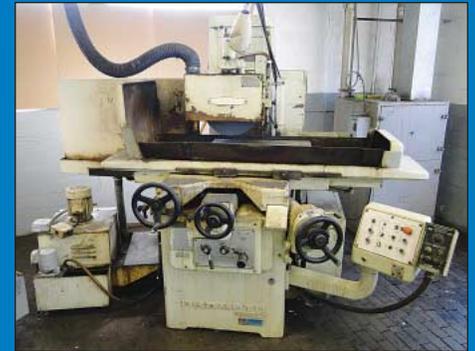
12" X 24" Okamoto Model Accugar-124N Hydraulic Surface Grinder
