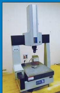
Brown and Sharpe Model Micro-Val Bench Type Coordinate Measuring Machine
