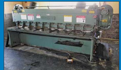
1/4" X 10' Cincinnati Model 1810 Mechanical Power Squaring Shear
