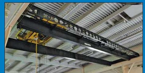
6 Ton X 40' Approx. Span Cleveland Tramrail Double Girder Top Running Overhead Bridge Crane
