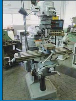
2 HP Bridgeport Variable Speed Vertical Milling Machine
