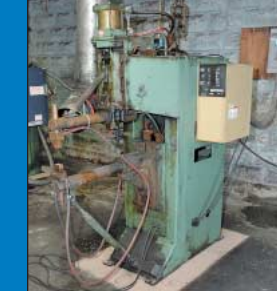
85 KVA Taylor-Winfield / Best Welder Model 77-268 Press Type Pneumatic Spot Welder
