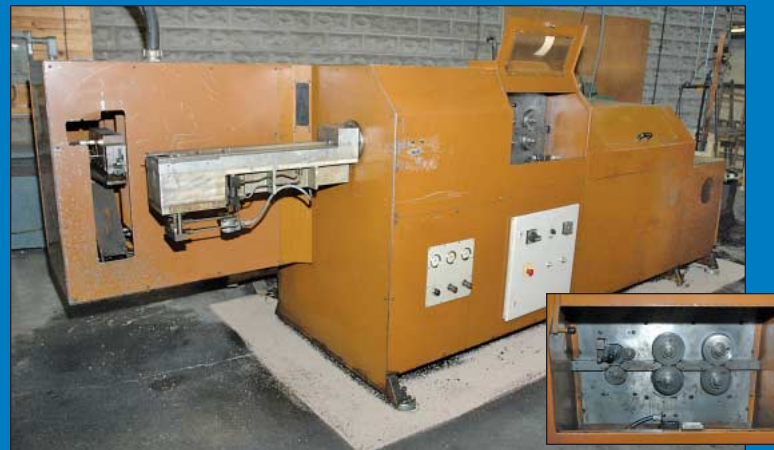
11 Ga. X 5/16" Cap. Pneuform Type & Machine No. PB-3A-690 CNC Wire Straightening Bending & Cutoff Machine
