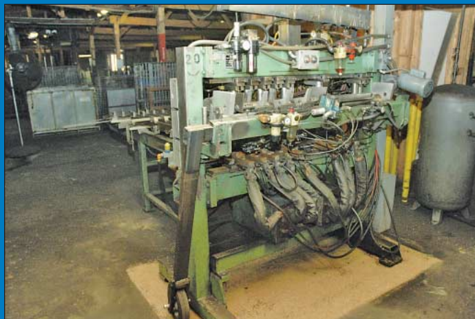
70 KVA Best Welder Model 85-117 Press Type Pneumatic Eight-Head Wire Mesh Welder
