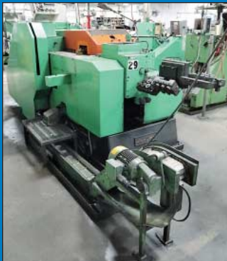
Asahi Okuma Model ORH-80 2-Die 3-Blow Cold Header
