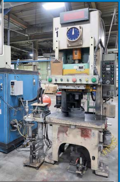
88-Ton & 66-Ton Seyi Clearing Presses Converted to Forge 12-Point Aircraft Engine Bolts
