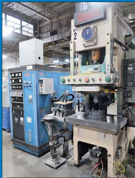
88-Ton & 66-Ton Seyi Clearing Presses Converted to Forge 12-Point Aircraft Engine Bolts
