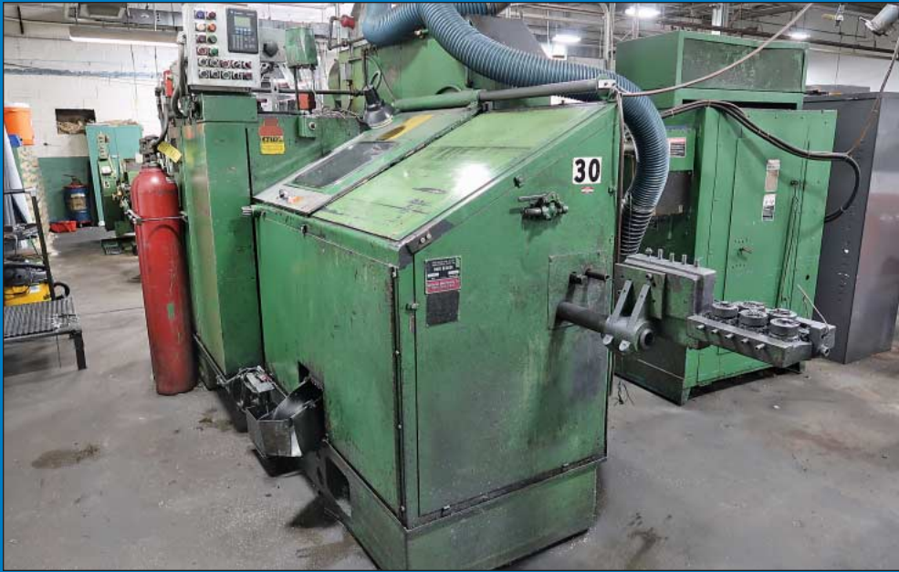
National Model 56HSL High Speed DSSD Cold Header Converted to Run Aerospace Fasteners Using Induction Heat
