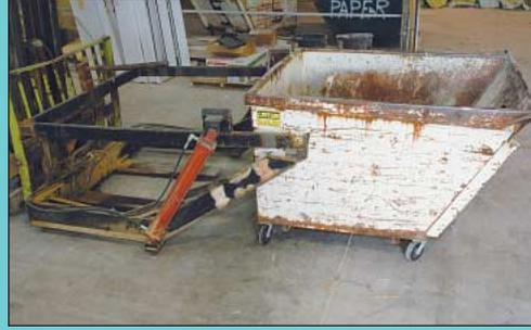
Mfg. Unknown Hydraulic Dump Hopper Dumper Forklift Attachment
