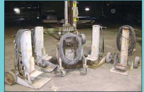
(4) 12 Ton Hydraulic House Jacks w/ 7-1/2 HP Electric Hydraulic Power Unit
