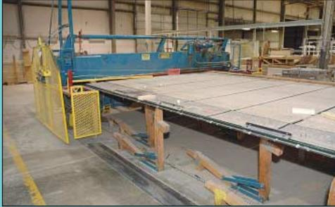
50 Ton Gang Nail Model Mark V Automatic Moving Truss Press
