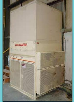
Unisol Model V34-E2-A Volu-Matic Insulation Blowing Machine
