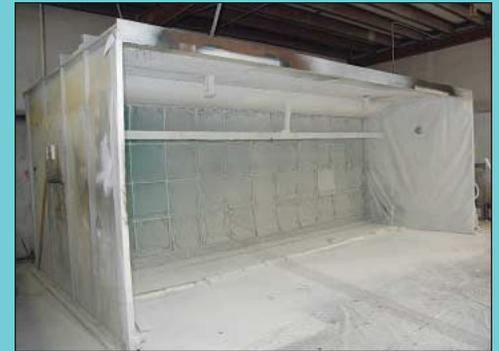
21' W X 8' D X 11' H Mfg. Unknown Bolt Together Rear Exhaust Galvanized Steel Paint Booth
