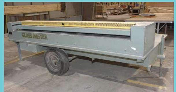
Class Master Model 215-3BT Groov-Master Duct Board Machine
