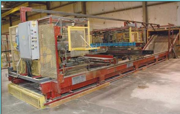
Timber Mill Model 6-20E Six-Blade Component Saw
