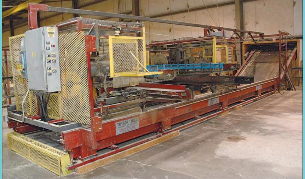
Timber Mill Model 6-20E Six-Blade Component Saw
