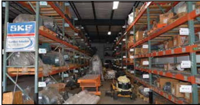
(29) Sections Tear Drop Pallet Racking
