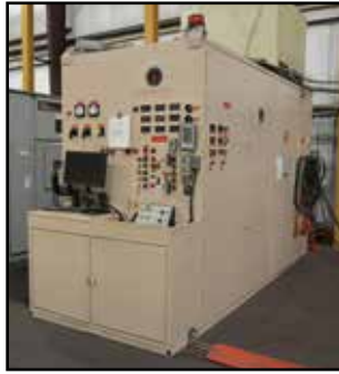
DYNAMOMETER w/MVC Solid State Soft Starter • KE 2,500 KVA Power Center • (2) JENKINS Power Meters • AW 2000-HP Load Tester & Table
