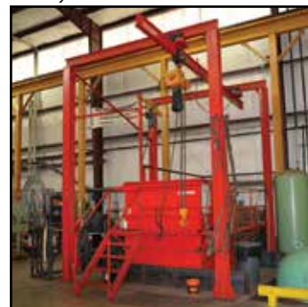
Custom Made Dip Tank w/Custom 4-Way Trolley Gantry System
