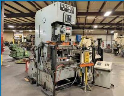
121 Ton Stamtec Model G1-110 Single Crank OBI Press
