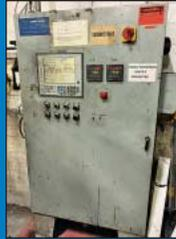
Control Panel for Plastisol Coating Machine
