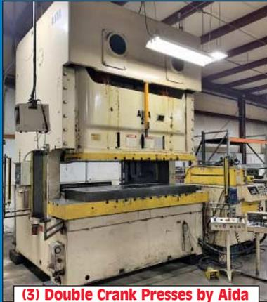
(3) Double Crank Presses by Aida and Stamtec to 275 Ton
