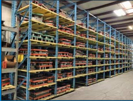
(28) Sections 4' x 4' x 188" High Heavy-Duty Adjustable Die Storage Rack System
