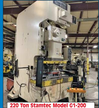
220 Ton Stamtec Model G1-200 Single Crank Gap Frame Press
