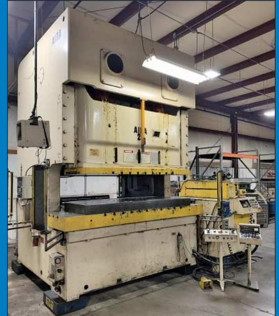
275 Ton Aida Model NC2-25(1) Double Crank Gap Frame Press
