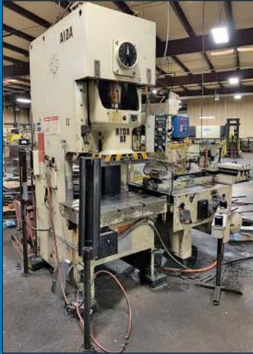
88 Ton Aida Model NC1-80(2) Single Crank Gap Frame Press
