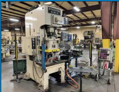
66 Ton Stamtec Model G1-60 Single Crank Gap Frame Press
