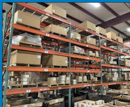
(50) Sections 42" x 108" x 15' High USP Adjustable Beam Pallet Rack
