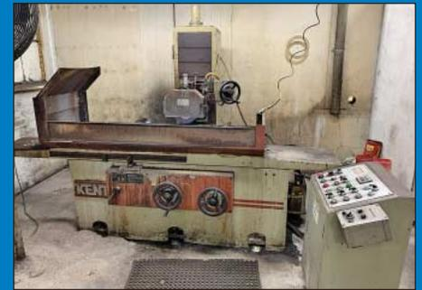
16" x 40" Kent Model KGS410AHD Hydraulic Surface Grinder
