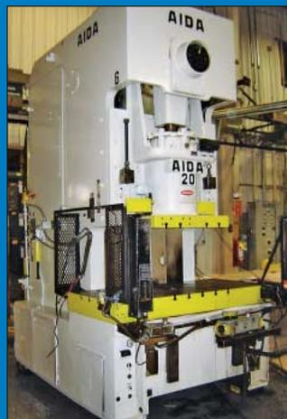
220 Ton Aida Model C1-20(1) Single Crank Gap Frame Press
