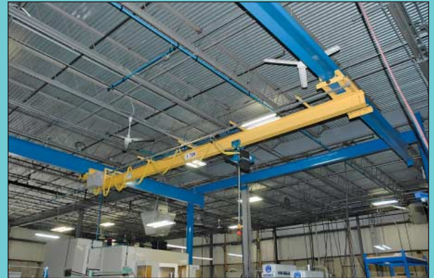
1 Ton X 30' Span X 40' Long X 15' High MHE Free Standing Bridge Crane System
