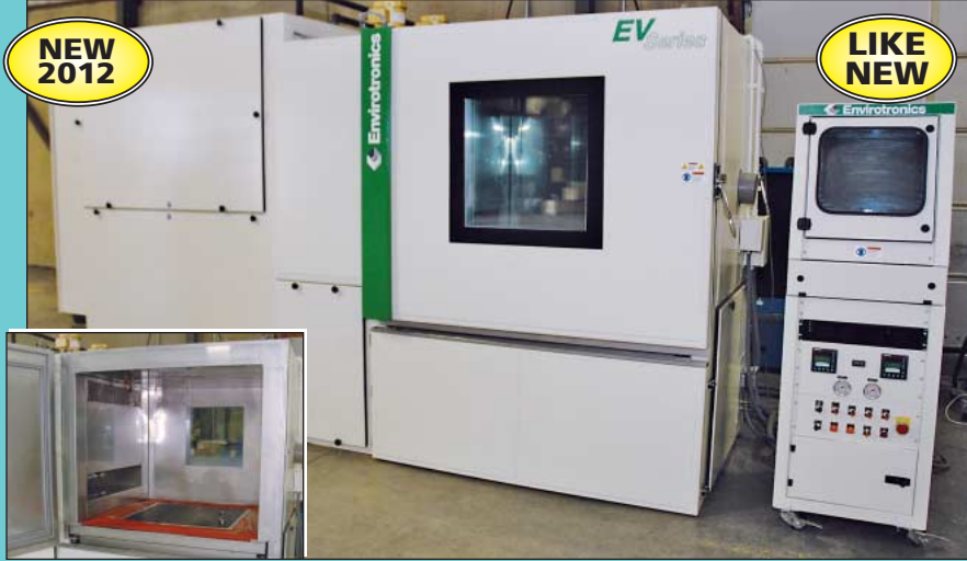
Envirotronics Model EVH1982-2-12-WC Temperature, Humidity, Vibration Environmental Test Chamber
