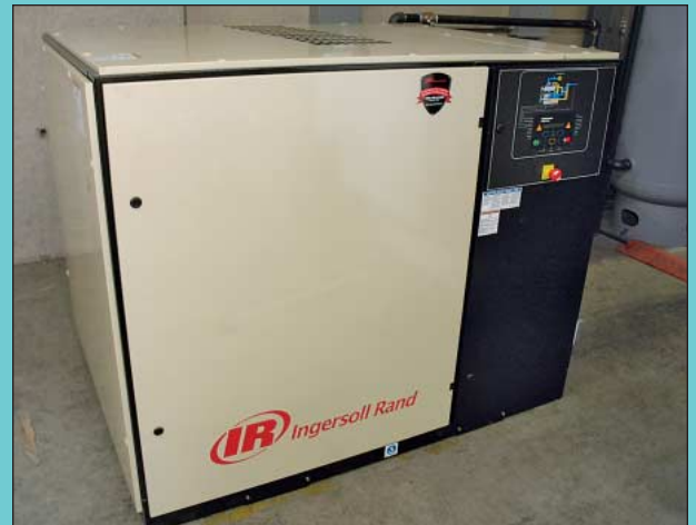
50 HP Ingersoll Rand Model UP6-50PE-125 Cabinet Enclosed Rotary Screw Air Compressor
