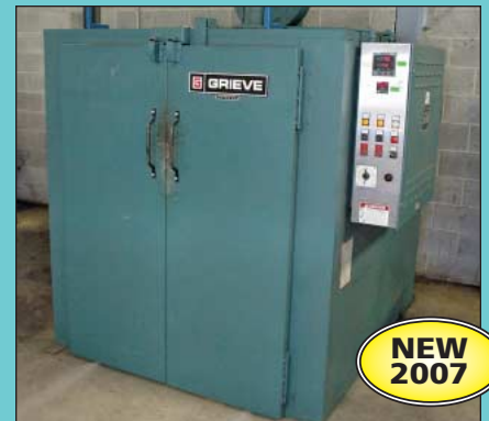
Grieve Model TBH-500 Electric Fired Truck Oven
