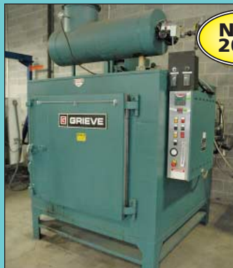
Grieve Model IC-1000 Natural Gas Fired High Temperature Inert Atmosphere Oven
