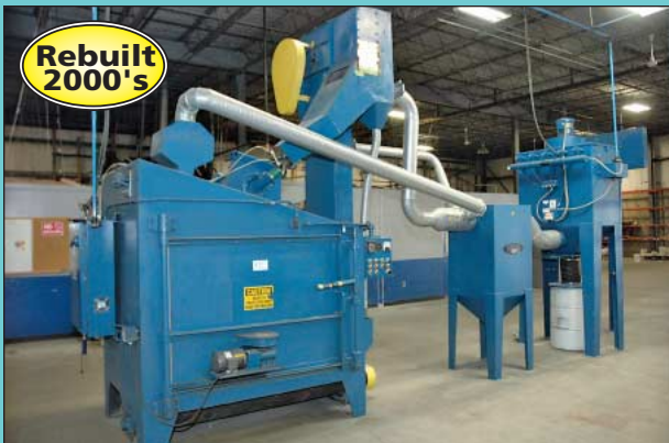
48" Dia. Abrasive Products Rotary Table Shot Blast Machine
