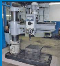
5' Arm X 11' Column Mazak Model Holemaster 5-12 Radial Arm Drill
