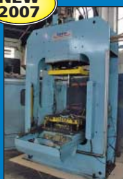
Serf Model AC080/600-025/410CP Decoring Machine
