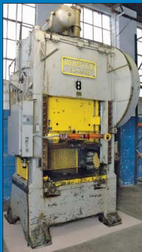
135 Ton Minster Model 50-6-48 Straight Side Double Crank Press
