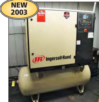
25 HP Ingersoll Rand Model UP-25-125 Rotary Screw Cabinet Enclosed Air Compressor
