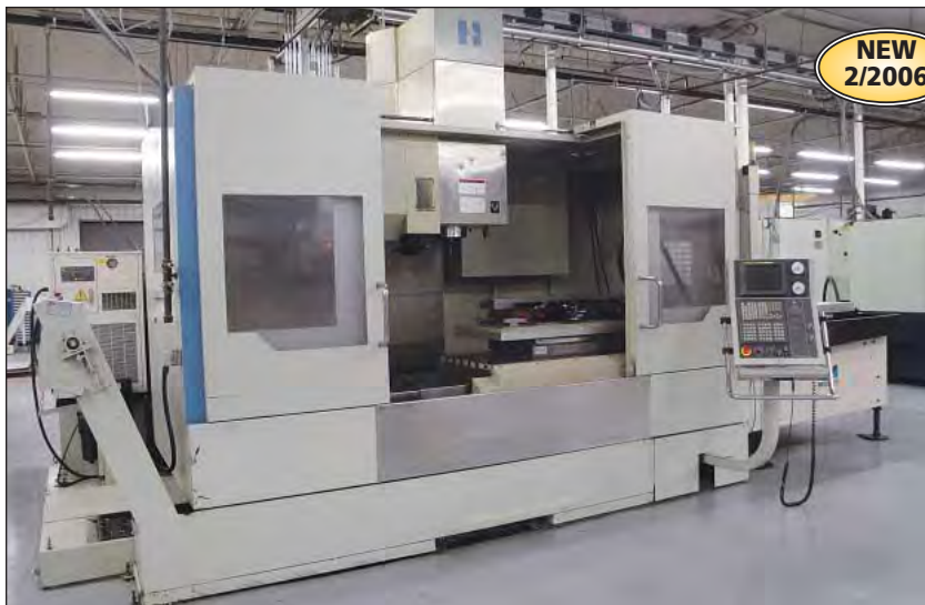
Hardinge Bridgeport Model VMC-1500XP3 HP Three-Axis CNC Vertical Machining Center w/ Midaco Pallet Changer
