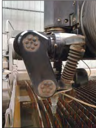
(2) Omax Model 80160 CNC Water Jet Cutting Tables
