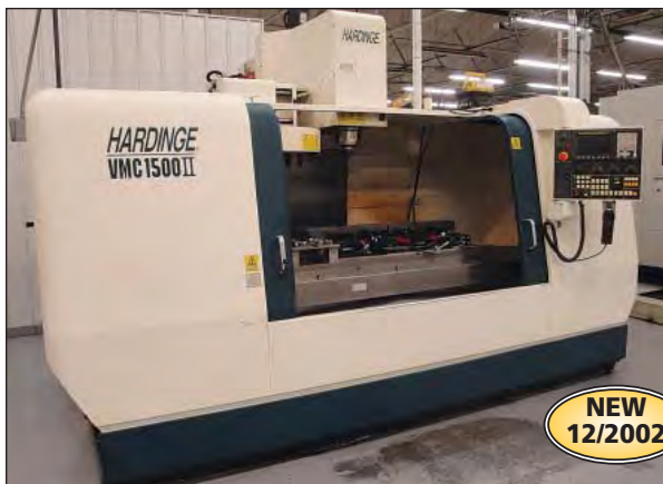
Hardinge Model VMC1500II Three-Axis CNC Vertical Machining Center
