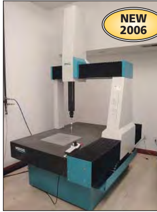
Wenzel Model LH87 CNC Bridge Type Coordinate Measuring Machine
