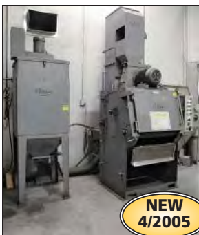
3 Cu. Ft. Gibson Model 3BB Rubber Belt Tumble Blast Machine
