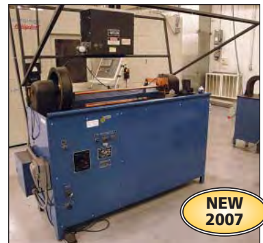
Magnaflux Model ARQ-545 Magnetic Particle Inspection System
