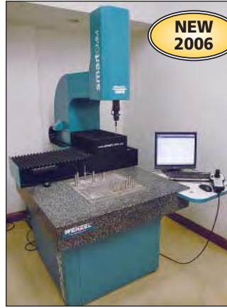
Wenzel Model Smart Cantilever Type Coordinate Measuring Machine
