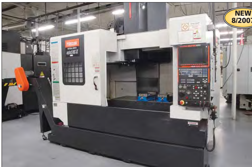
Mazak Model Nexus 510C-II Three-Axis CNC Vertical Machining Center
