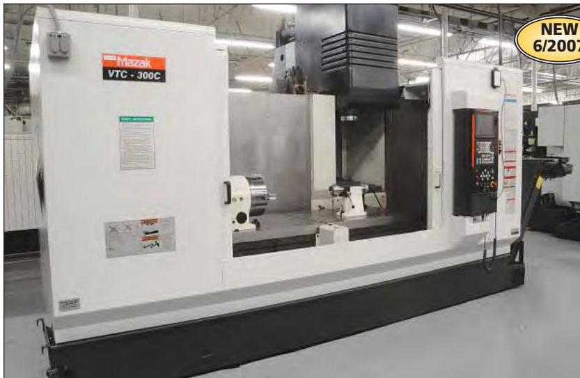
Mazak Model VTC-300C Three-Axis CNC Trailing Column Vertical Machining Center
