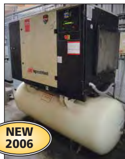
25 HP Ingersoll Rand Model UP6-25-125 Rotary Screw Cabinet Enclosed Heat Treat Air Compressor w/ Integrated Air Dryer
