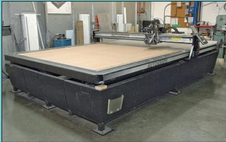
Cybernation Autograph Multi Cutter 8000 Three-Axis CNC Sign Router
