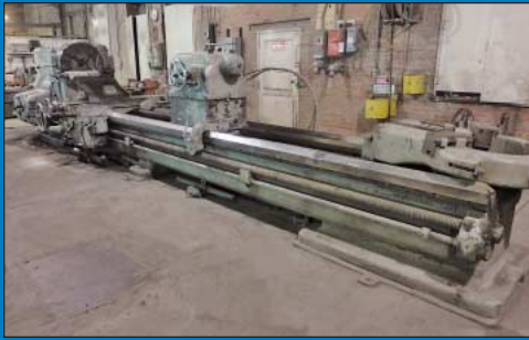
40" X 204" American Pacemaker Style J-6 Geared Head Engine Lathe
