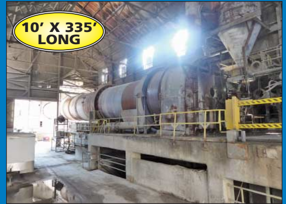
11'-3" Dia. Discharge / 10' Dia. Feed End X 335' Long (K-1) Vulcan Rotary Kiln System
