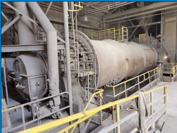
Nordberg 9' Dia. X 34' L Steel Drum Two-Compartment Finish Mill
