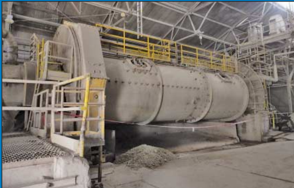
Nordberg 9'6" Dia. X 34' L Steel Drum Two-Compartment Raw Mill
