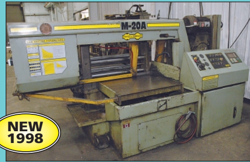
20' X 30' Hyd-Mech Model M-20A Automatic Horizontal Band Saw
