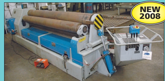
**33/64" X 8' Waldemar Model K-11-8 Hydraulic Power Plate Bending Roll
