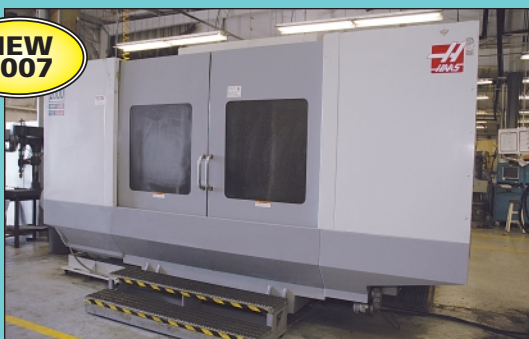
Haas Model EC-2000 CNC Horizontal Machining Center
