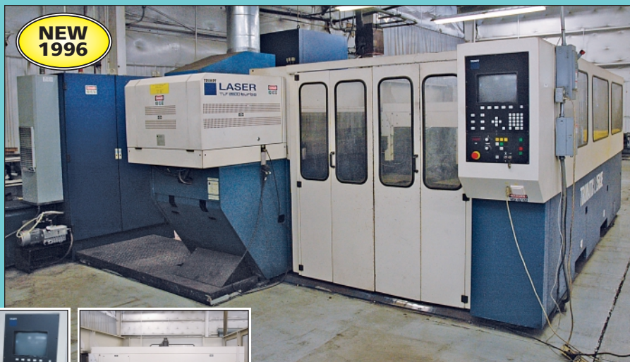
2,600 Watt Trumpf Model Trumatic L2503E Laser Cat CNC Laser Cutting Machine
