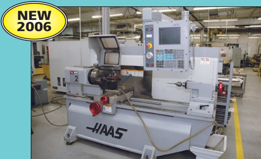
Haas Model TL-2 CNC Toolroom Lathe
