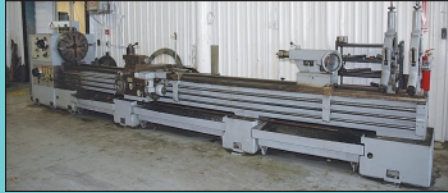
28" X 204" Summit Model 28 Geared Head Engine Lathe
