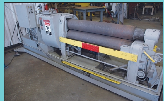
1/4" X 4' Webb Model R3LR8004 Mechanical Power Plate Bending Roll
