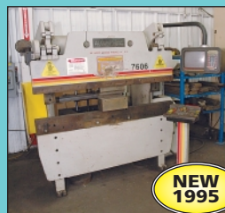
60 Ton X 6' Accurpress Model 7606 CNC Hydraulic Press Brake w/ CNC Backgauge
