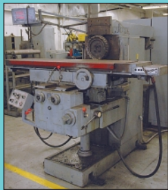
Induma Model 2045P Horizontal Milling Machine
