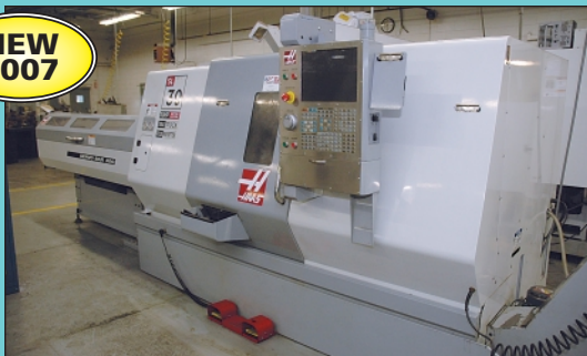
Haas Model SL-30T Slant Bed CNC Turning Center
