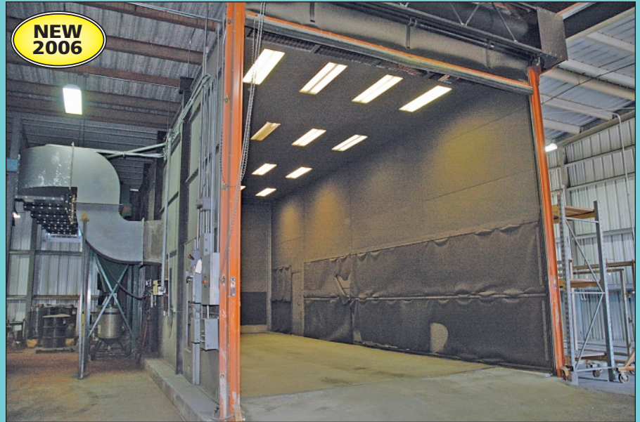
16' Wide X 40' Long X 17' High Carolina Virginia Model 17-16-20 Industrial Blast Drive-In Shop Blast Room
