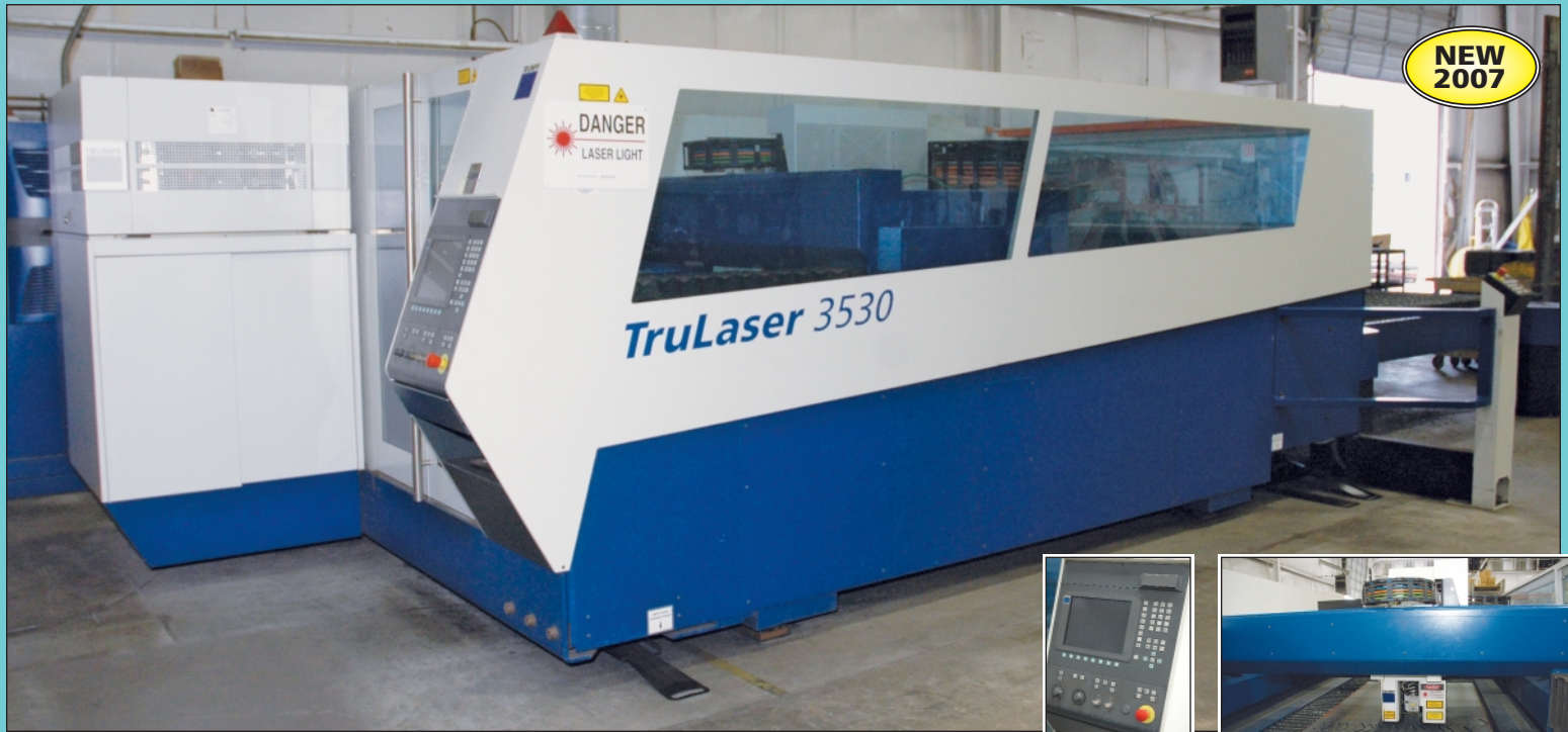
4,000 Watt Trumpf Model TruLaser 3530 CNC Laser Cutting Machine
