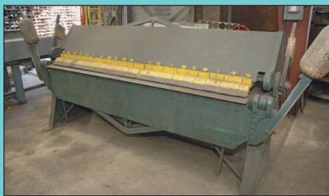
8' Chicago Model BPO-812-6 Manual Finger Brake
