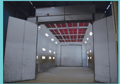
20' Wide X 40' Long X 16' High Mfg. Unknown Cross Draft Drive-Thru Paint Booth
