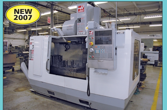
Haas Model VF-3B CNC Vertical Machining Center
