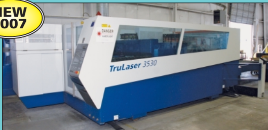
4,000 Watt Trumpf Model TruLaser 3530 CNC Laser Cutting Machine
