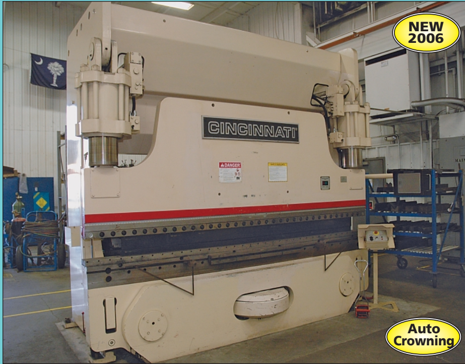
350 Ton X 12' Cincinnati Model 350PFX10 Proform CNC Hydraulic Power Press Brake w/ Auto Crowning & CNC Backgauge
