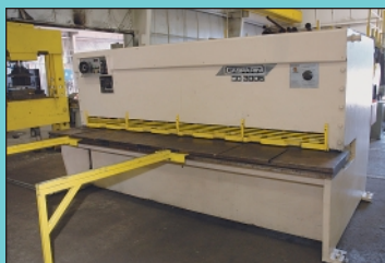
5/16" X 10' Gasparini Model CO3006 Hydraulic Power Squaring Shear
