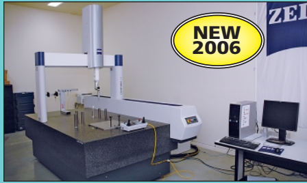
Zeiss Model Contura G2/10/21 RDS Coordinate Measuring Machine
