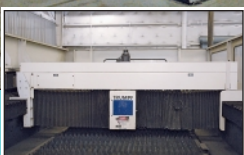
2,600 Watt Trumpf Model Trumatic L2503E Laser Cat CNC Laser Cutting Machine
