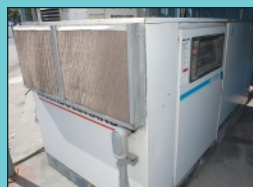
75 HP Ingersoll Rand Model SSR-EP75 Cabinet Enclosed Rotary Screw Air Compressor
