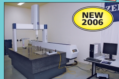
Zeiss Model Contura G2/10/21 RDS Coordinate Measuring Machine
