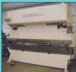
225/150 Ton X 12' Niagara Model 1B-150-10-12 Mechanical Power Press Brake w/ CNC Backgauge
