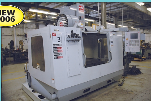
Haas Model VF-3BYT CNC Vertical Machining Center
