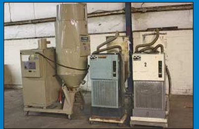
Plastic Auxiliary Equipment Including Dryers
