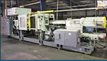
(3) 500 Ton x 60 Oz. Van Dorn Model 500H-RS-60F-CV Hydraulic Clamp Injection Molding Machines
