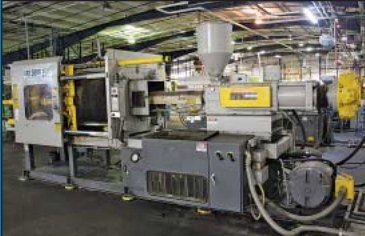
350 Ton x 30 Oz. Van Dorn Model 350-RS-30F-VV Toggle Clamp Injection Molding Machine
