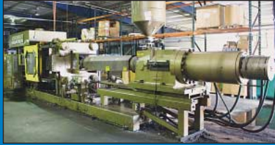
700 Ton x 225 Oz. Cincinnati Milacron Model 700-225 Hydraulic Clamp Injection Molding Machine
