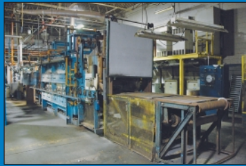
30" Wide General Electric Glo-Bar Continuous Mesh Belt Type Brazing & Annealing Furnace
