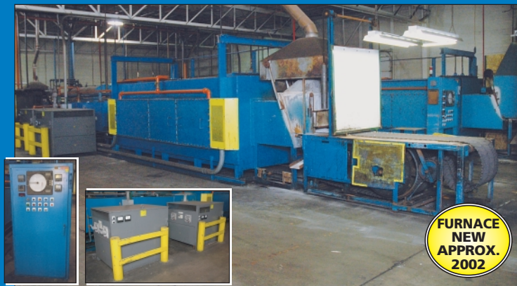
24" Wide Lo-Temp Brazing Co. Electric Continuous Mesh Belt Brazing & Annealing Furnace
