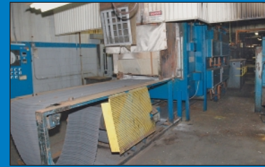
24" Wide Westinghouse Electric Glo-Bar Continuous Mesh Belt Brazing & Annealing Furnace
