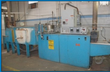
6" Wide CI Hayes Inc. Electric Continuous Mesh Belt Brazing & Annealing Furnace
