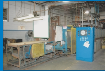
24" Wide General Electric Glo-Bar Continuous Mesh Belt Type Brazing & Annealing Furnace
