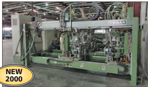
Urban Model SV-800/2.5M Four-Point Window Frame Corner Cleaner
