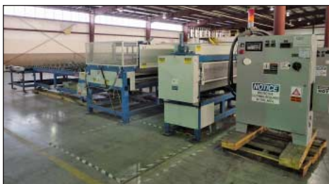
(5) 84" GED Model MHMO3500416R 76.8 KVA Insulated Glass Oven / Roll Press Systems
