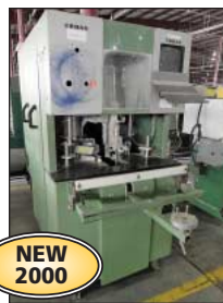
Urban Model SV-500 Single Point Window Frame Corner Cleaner
