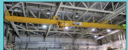
10 Ton x 75' (Approx.) Span Crane Hoist Engineering Co. Bottom Running Overhead Bridge Crane
