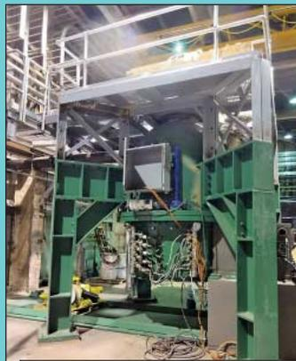
96" Dia. x 96" Wide (Approx.) Vacuum Chamber; Components and Controls
