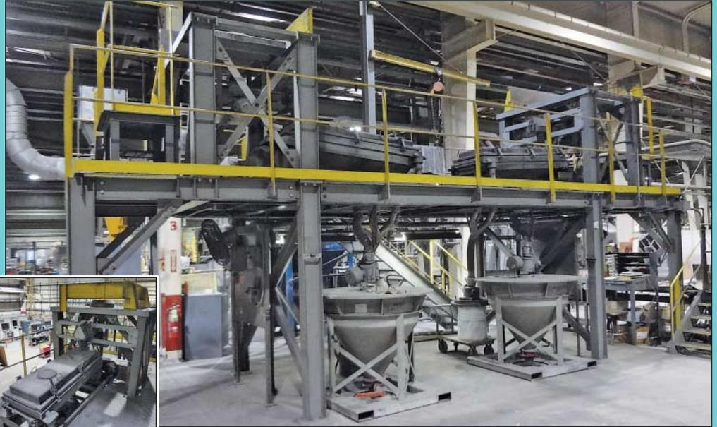
(2) 20" x 62" Rotex Platform Mounted Screeners w/ Erez Magnet Systems
