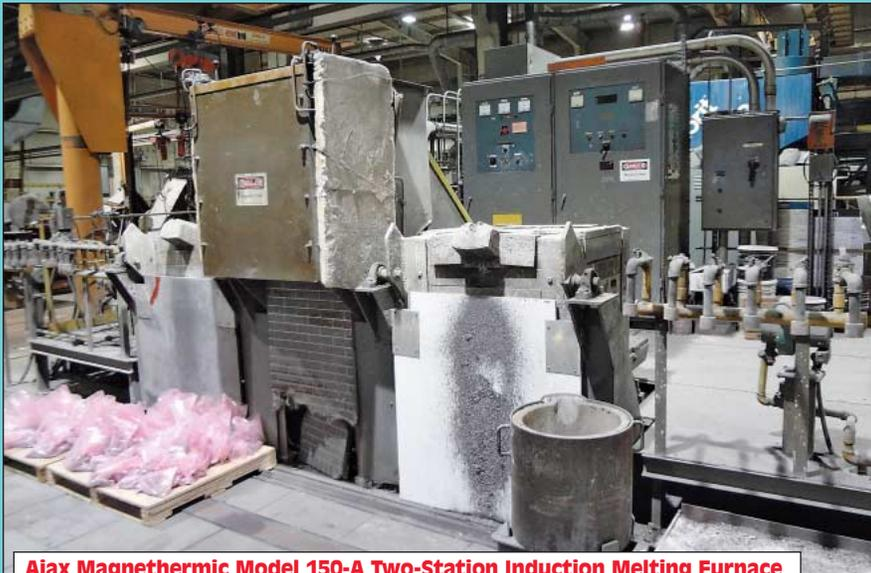
**Ajax Magnethermic Model 150-A Two-Station Induction Melting Furnace**
