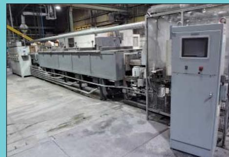
(2) 100 KW Spang Type KO5409-1 5-Zone E-Core Belt Type Annealing Furnaces
