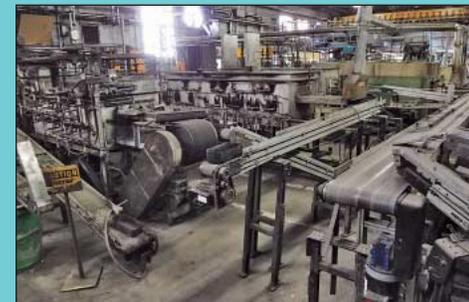
Spang Type K-5178 3-Zone Electric Belt Type Annealing Furnace
