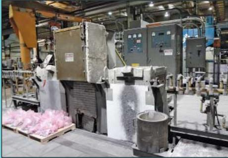
Ajax Magnethermic Model 150-A Two-Station Induction Melting Furnace
