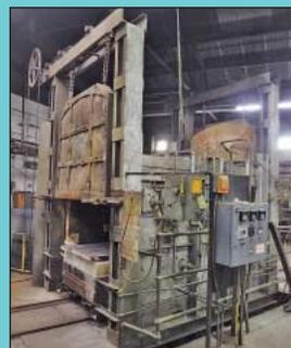
Eclipse Fuel and Engineering Gas Fired Car Bottom Furnace
