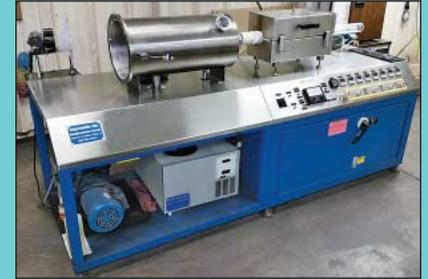
Paratronix Model 1092 Horizontal Parylene Coating Machine
