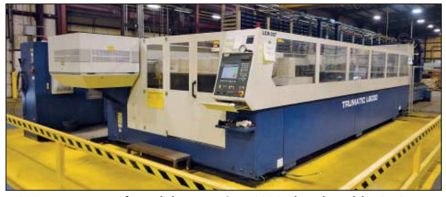
4,000 Watt Trumpf Model Trumatic L-6030 Shuttle Table CNC Laser
