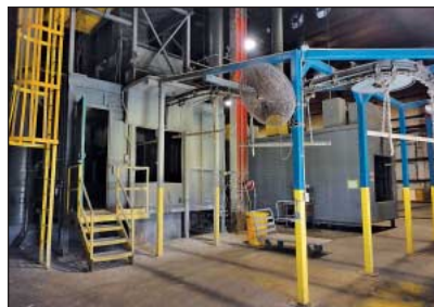
Small Parts Line Consisting of Pass-Thru Washers, Ovens, Pass-Thru Paint Booth, Conveyor and Related
