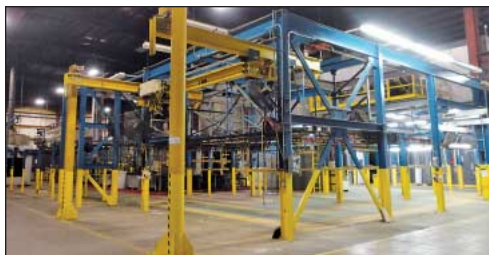
Heavy Duty Channel Overhead Conveyor System w/ Approx. 25' Wide Racks, Approx. 25' On Centers (Large Part E-Coat Line)
