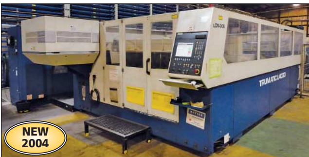
4,000 Watt Trumpf Model Trumatic L-4030 Shuttle Table CNC Laser
