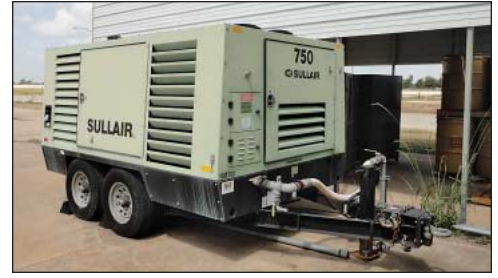
Sullair Model 750 Cat Industrial Duty Diesel Power Air Compressor
