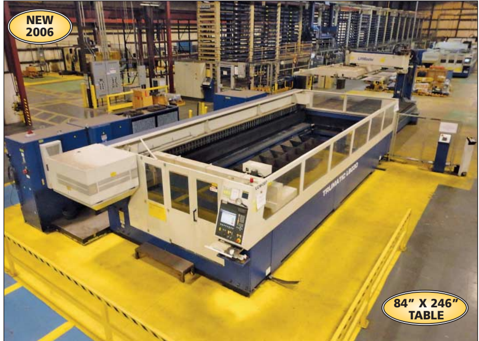
4,000 Watt Trumpf Model Trumatic L-6030 Shuttle Table CNC Laser (Elevated View)
