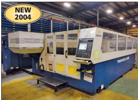
4,000 Watt Trumpf Model Trumatic L-4030 Shuttle Table CNC Laser
