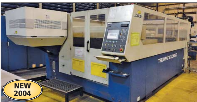
(2) 4,000 Watt Trumpf Model Trumatic L-3030 Shuttle Table CNC Lasers
