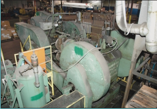
3/4" Manville Model 500-C Two-Blow Double End Rod Header
