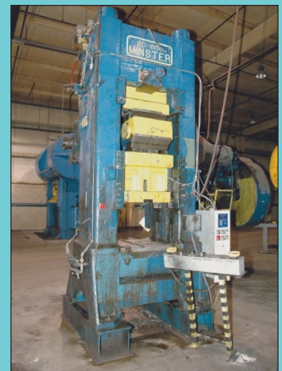
600 Ton Minster Model 90-600 Knuckle Joint Press
