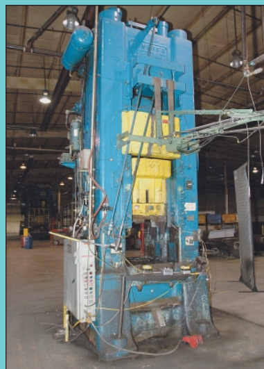
1,000 Ton Minster Model 90-1000 Knuckle Joint Press
