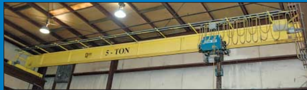
(2) 5 Ton X 50' Span Odom Industries Top Running Single Girder Overhead Bridge Cranes
