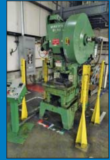
32 Ton Minster Model B1-32 High Speed Gap Frame Press
