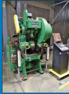
35 Ton South Bend Model 35-FW-AC OBI Press
