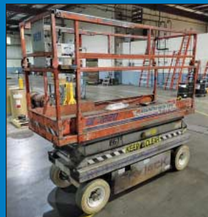
Skyjack Model 3220 Electric Scissor Lift
