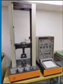
Instron Model 1122 Tensile Tester w/ Break Detector
