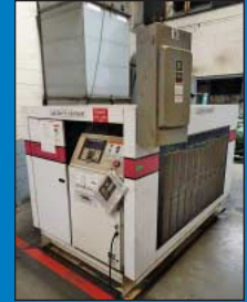
100 HP Gardner Denver Model EBPMC Cabinet Type Air Compressor
