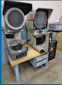
16" Deltronic Model DH216 Optical Comparator w/ Deltronic MPC-5 DRO
