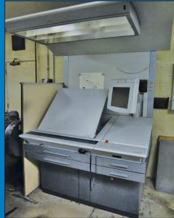
Heidelberg Control Console
