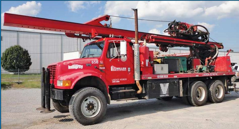
2002 Versa Drill Model Versa Sonic Drill w/ Sonicator 50K Drill Head on 2002 International Navistar 4900 6X6 All Wheel Drive Truck
