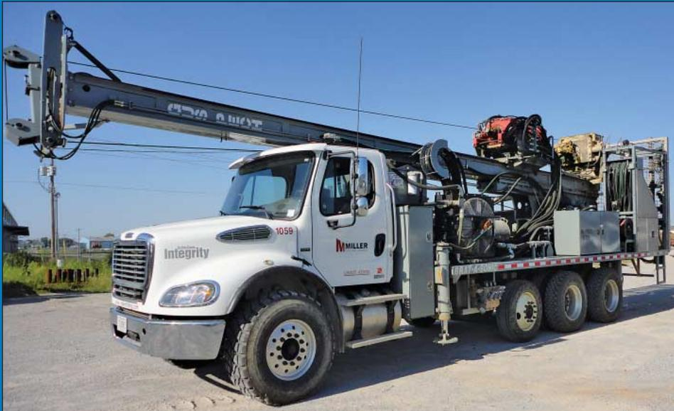
2008 Gus Pech Model GP-26-400RD Super Sonic II Drill w/ Sonicator 50K Drill Head on 2008 Freightliner M2 112 T/A Business Class Drill Truck
