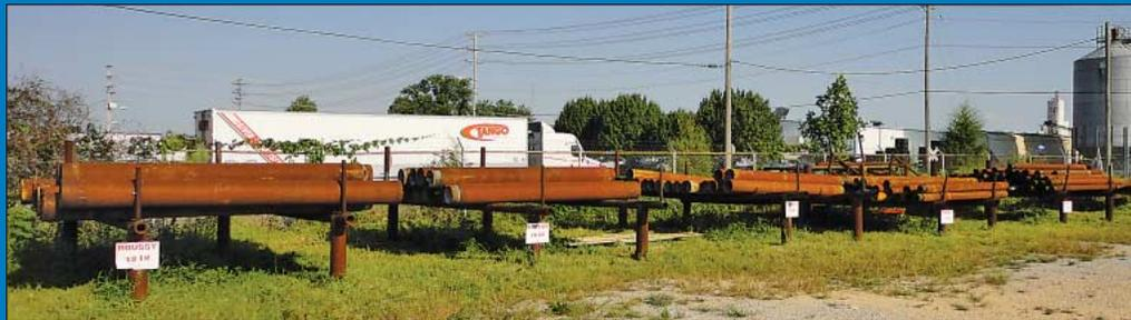
Approx. 1,650' Sonic-Roussy Thread Drill Pipe From 3-1/2" To 12-3/4" Diameter
