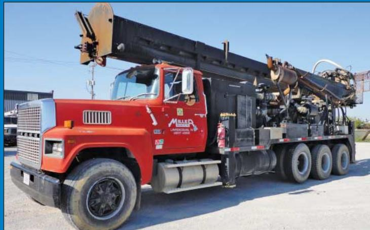
6,656 Approx. Rig Hours, Sonoric Model 50K Sonic Drill Head, 23,000 Lbs. Hoist Capacity, 12,000 Lbs. Winch Over Jib, 2,000 Lbs. Auxiliary Winch Over Jib, Hydraulic Rod Spinner, 37 GPM Bean Pump, Head Recently Rebuilt **SEE PHOTO**
