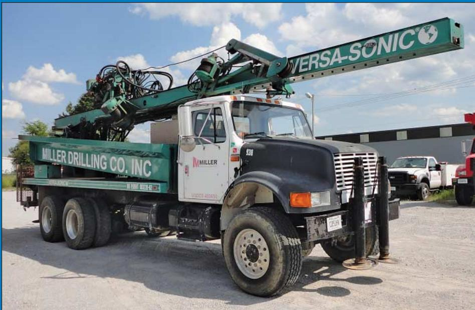
2002 Versa Drill Model Versa Sonic Drill w/ Sonicator 50K Drill Head on 2002 International Navistar 4900 6X6 All Wheel Drive Truck
