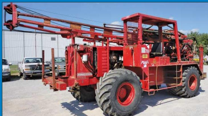
CME Central Mine Equipment Model 750X Drill on 2000 CME Rubber Tire All Terrain Vehicle
