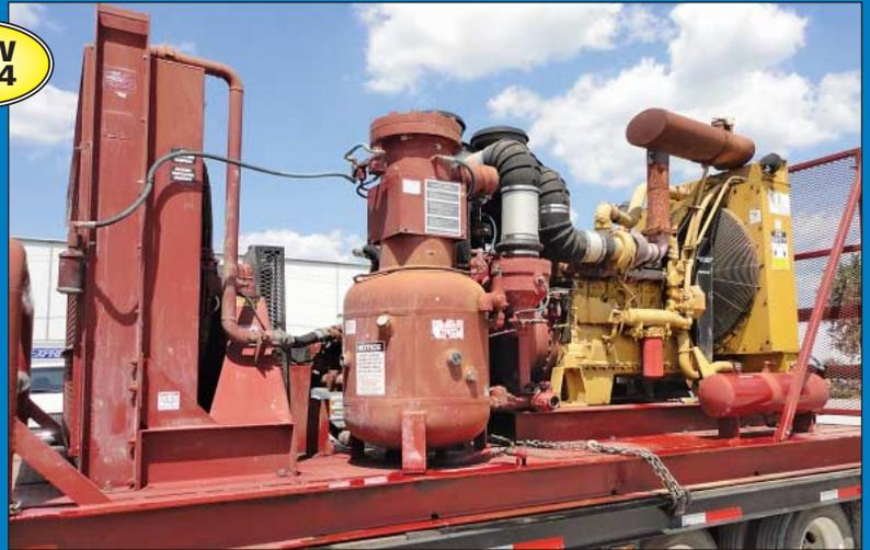
2004 – 630 HP Keystone Drill Services Unit No. KC-3 Sullair / Caterpillar Skid Mounted Diesel Powered Air Compressor
