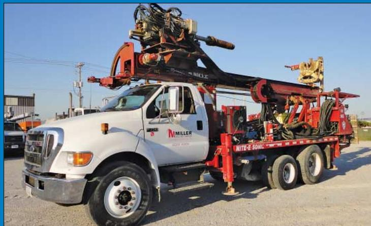
2005 Gus Pech Model Mite-E-Sonic Drill w/ Sonoric 50K Drill Head on 2005 Ford F-750 S/A Truck
