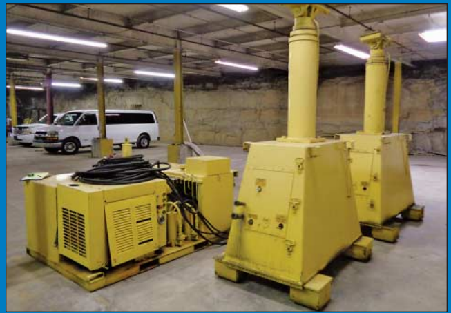
200 Ton Lift Systems Model 2200 Two-Post Self Propelled Gantry System
