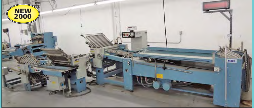
30" X 50" MBO Model B-30-1-30 4-Plate Continuous Feed Folder w/ 8 and 16-Page Attachments
