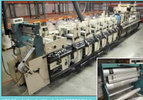
16" Mark Andy Model 41368816Y-A Six-Color Flexographic Printing Press
