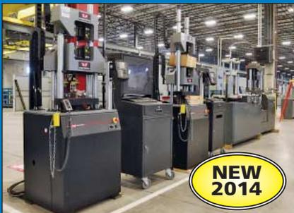
(2) 300-KN Instron Model 300DX-C3A-G7E Dual Tension and Compression Testers
