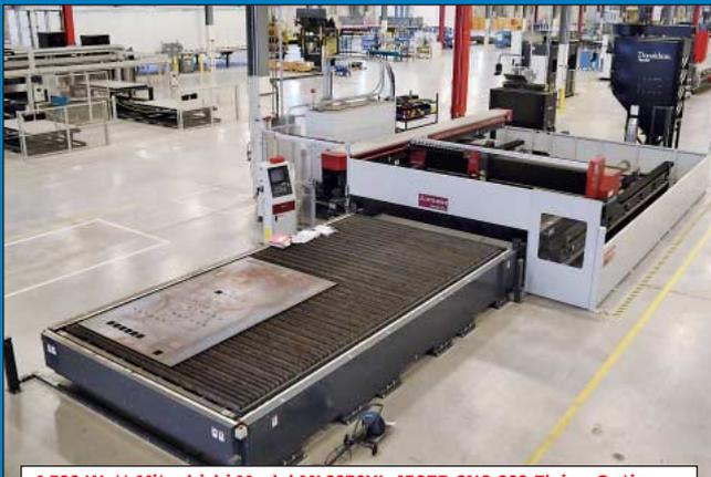
**4,500 Watt Mitsubishi Model ML6030XL-45CFR CNC CO2 Flying Optic Laser**
