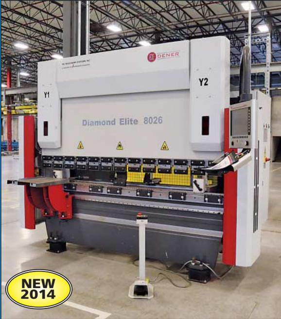
**(2) 88 Ton X 102" Dener Model DE80-26-AC-ZL-2M Multi-Axis CNC Press Brakes**
