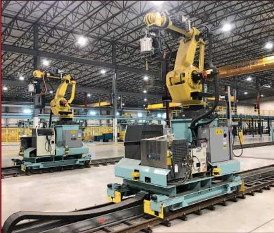
**(2) Genesis / Fanuc Track-Travelling Single-Robot Spot Welding Systems**
