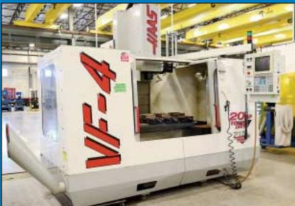
Haas VF-4 CNC Vertical Machining Center
