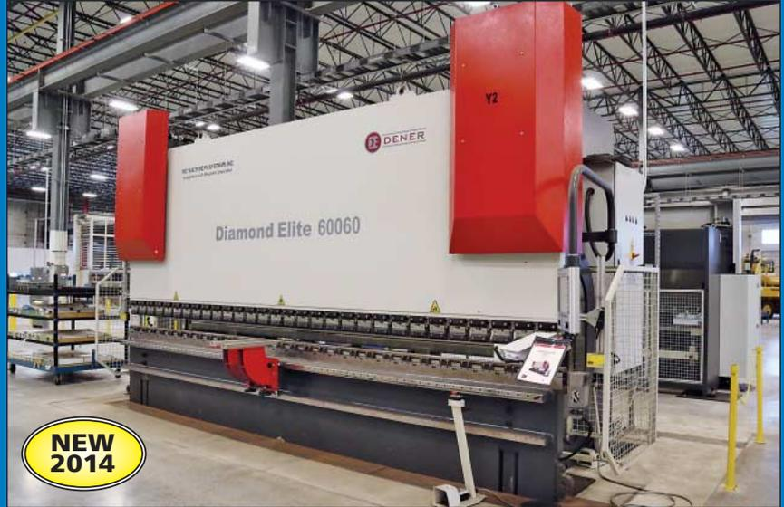
**660 Ton X 238" Dener Model DE600-60-AC-ZL-2M Multi-Axis CNC Press Brake**
