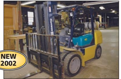
7,000 Lb Komatsu Model FG40ZT-7 Pneumatic Tire LP Gas Lift Truck
