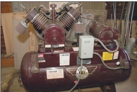
15 HP Quincy Model 2153D12HCA Horizontal Tank Two-Stage Air Compressor
