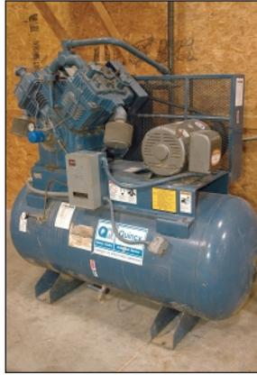
25 HP Quincy Model QR5120EST Two-Stage Horizontal Tank Rotary Screw Air Compressor
