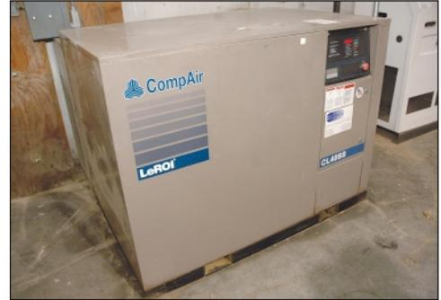
40 HP LeRoi Model Compair CL405S Cabinet Type Rotary Screw Air Compressor
