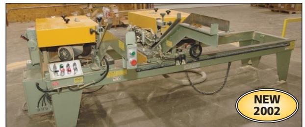
Ruvo Triad Model 855 Fully Automatic Hopper Feed Casing, Mitre & Kerf Saw
