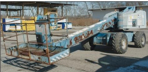
Genie Model S60 Pneumatic Tire LP Gas Snorkel Type Boom Lift
