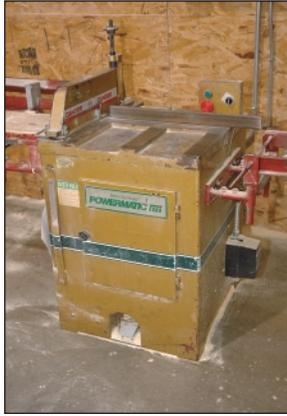
14" Powermatic Model MMM Upacking Cut-Off Saw
