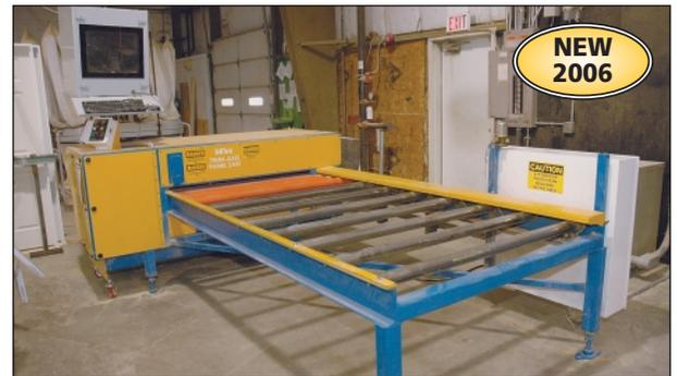
MiTek Twin-Axis CNC Panel / Sheathing Saw
