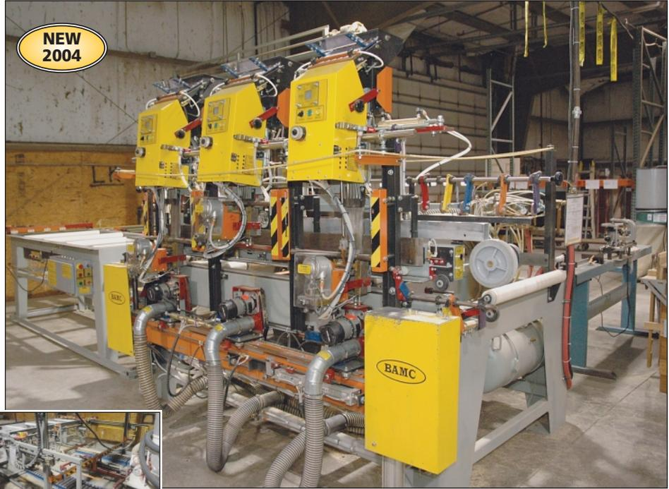
BAMC Builders Automation Machinery Co. Model 625/1550 REM Automatic Pre-Hung Door Machine
