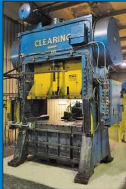
**135 Ton Clearing Straight Side Double Crank Press**
