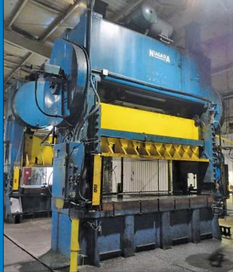
**260 Ton Niagara Model S2-260-120-60 Straight Side Double Crank Press**
