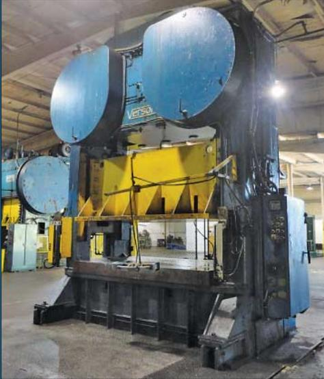
**250 Ton Verson Model Co. C2-250-108-60T Straight Side Double Crank Press**
