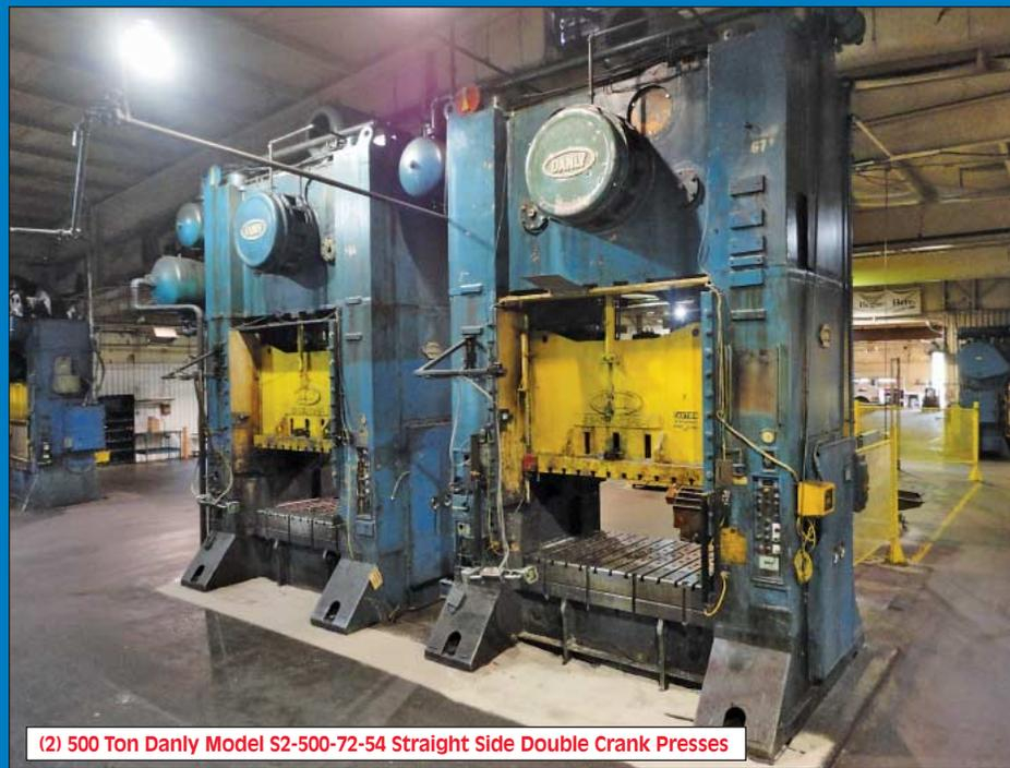
**(2) 500 Ton Danly Model S2-500-72-54 Straight Side Double Crank Presses**
