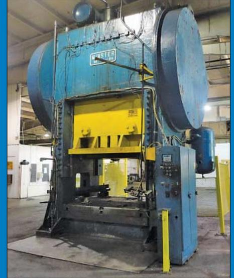
**700 Ton Minster Model 50-11-84 Straight Side Double Crank Press**
