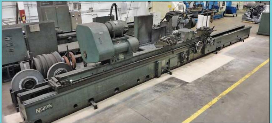
24" x 192" Norton Combination Crankshaft and O.D. Cylindrical Grinder
