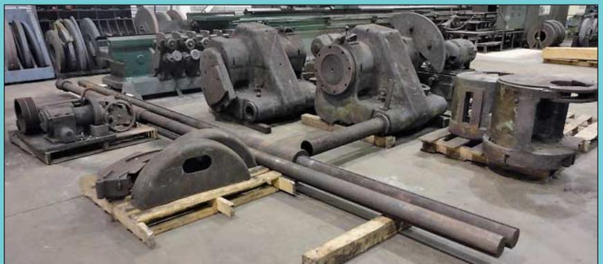
(2) Pot Chuck Heads for Cranks Shafts
