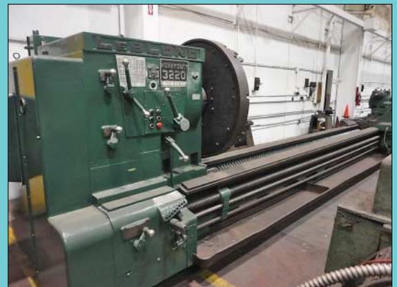
54" x 246" Leblond Model 3220 Heavy Duty Engine Lathe
