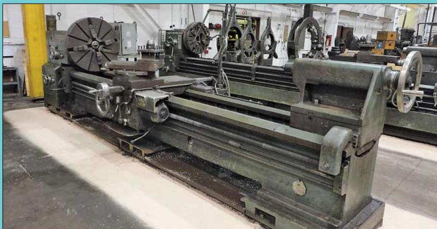
38" x 130" Sirco Model PA-36 Engine Lathe
