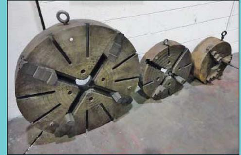
Large Quantity Lathe Tooling
