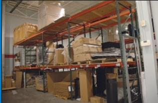
(52) Sections 48" Deep X 96" - 144" Wide X 12' High Adjustable Beam Pallet Rack
