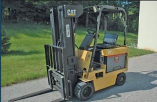
3,000 LB Caterpillar Model M50SA Sit Down Electric Lift Truck
