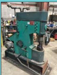
Sayha Model SSM-50 Powered Forging Hammer
