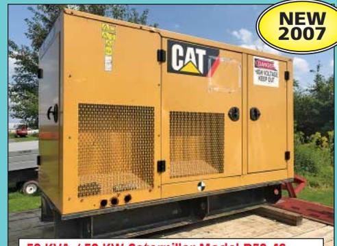
50 KVA / 50 KW Caterpillar Model D50-4S Generator Set
