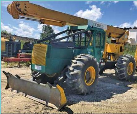
Timberjack Model 240B Cable Std / Shift Articulating 4-Wheel Drive log Skidder
