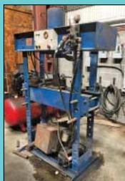
50 Ton Sayha Model SHP-50 Hydraulic H-Frame Press
