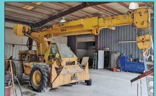
Galion Model 150-A 4-Wheel Drive Rubber Tire Hydraulic Crane
