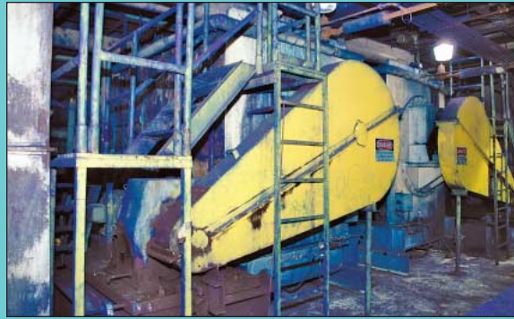
(2) 300 Cubic Foot Jacketed Stainless Steel Ribbon Blenders
