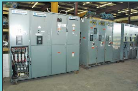
Allen Bradley Centerline Motor Control Center Starter Panel, 4,160 Volt, 900 HP, with 12 Motor Starter
