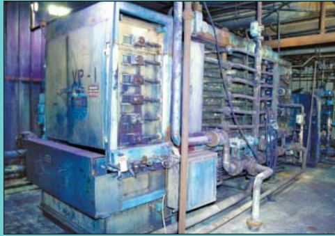
(2) Filtra Systems Stainless Steel Verti-Presses or Dry Caking Presses
