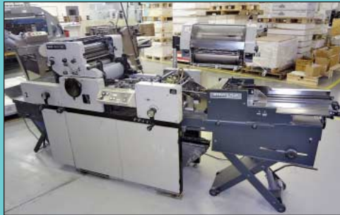
13" X 18" Itek Model 3985 Two-Color Offset Press w/ Strate Flo Envelope Feeder
