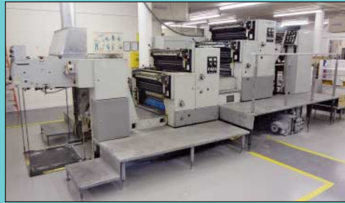
30" X 29" Omcsa Model H426-N Four-Color Offset Press
