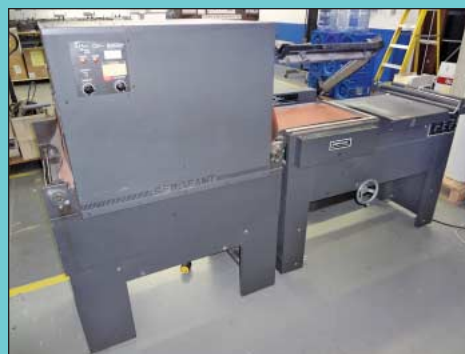
14" X 20" Sergeant Model LSLRSMPLS III "L" Sealer w/ Shrink Tunnel
