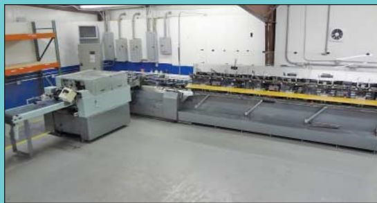
Macey Model 542-6 Six-Station Saddlebinder Stitching Line
