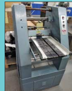
14" Rollem Auto 4 Perforator / Scoring Machine
