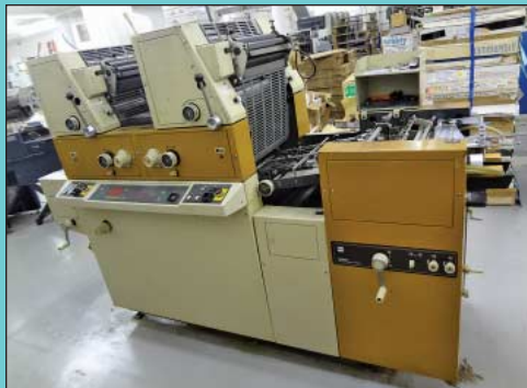
12" X 17" Multigraphic Model 1650MC Two-Color Offset Press
