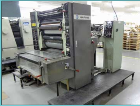
25" X 29" Harris Model L129C Single-Color Offset Press
