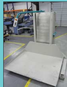
40" X 50" Perfecta Model SL12-P Electric / Hydraulic Paper Lift
