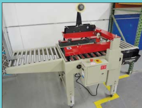
"K" Master Model CSM-5000 Carton Taper / Sealer
