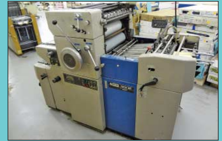
14" X 18" Ryobi Model 480K-NP Single-Color Offset Press w/ Score, Perforating, & Numbering
