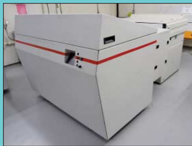
Escher-Grad Inc. Model EG-8200 Series Image Setter
