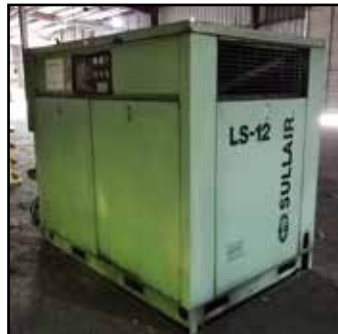
SULLAIR LS-12 60-HP Air Compressor
