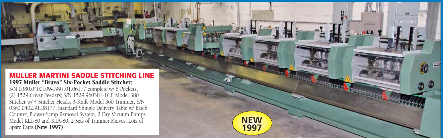
1997 Muller "Bravo" Six-Pocket Saddle Stitcher - Overall View
