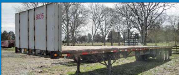
48' - 80' 1998 Great Dane Model GPES248-80 Extendable Steel Deck Tandem Axle Trailer
