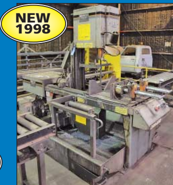
18" HEM Model V100LM-2 Semi-Auto Tilt Frame Vertical Band Saw
