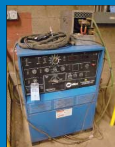
350 Amp Miller Model Syncrowave 350 TIG Welder
