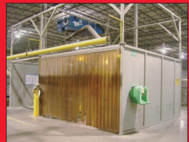
15' X 24' Bolt-Together Welding Enclosure
