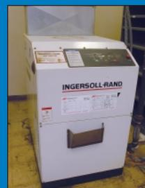
25 HP Ingersoll Rand Model SSR-EP255E Cabinet Type Rotary Screw Air Compressor
