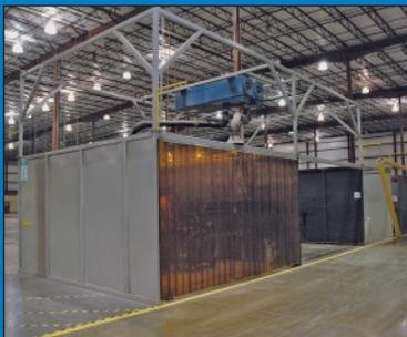
15' X 40' Bolt-Together Welding Enclosure
